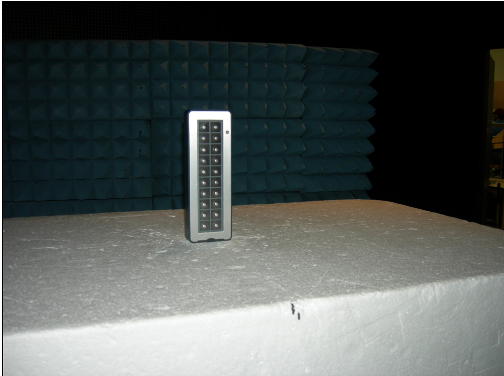
Figure 3: Radiated Emissions – YPOS
