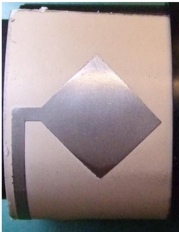
Top conformal antenna
