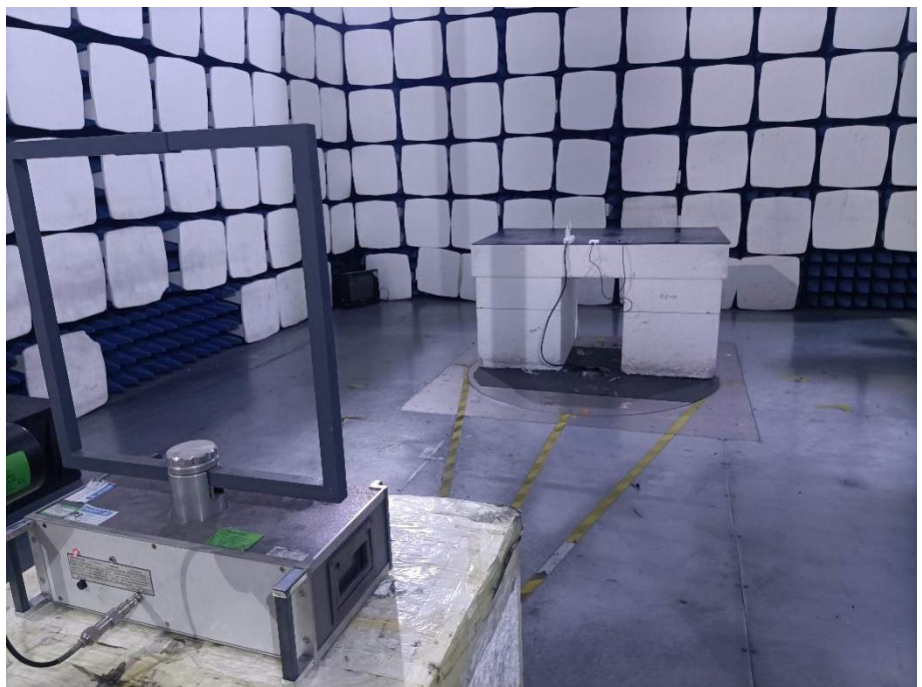
Radiation Emission Test Setup (Below 30MHz)
