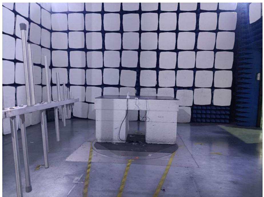
Radiation Emission Test Setup (30MHz to 1GHz)
