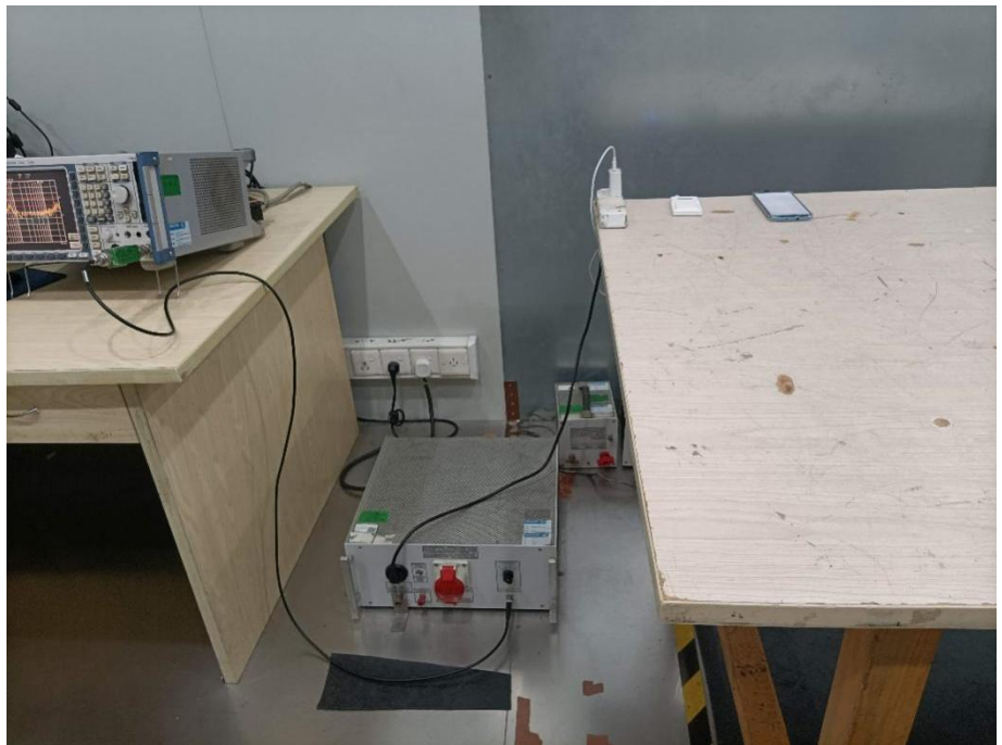
Conducted Emission Test Setup
