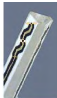
Figure 3.3 Probe Thick-Film Technique
