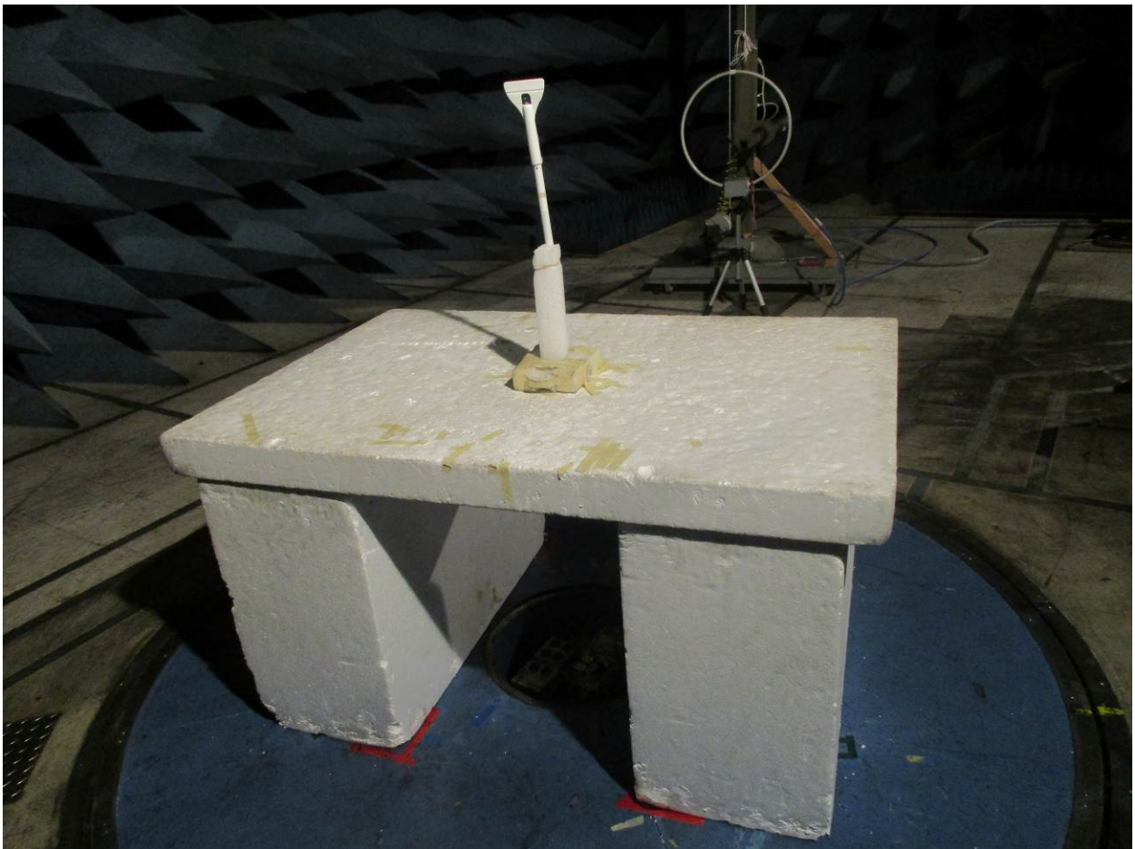
Figure 2: Radiated Emissions – Back View – 9 kHz – 30 MHz
