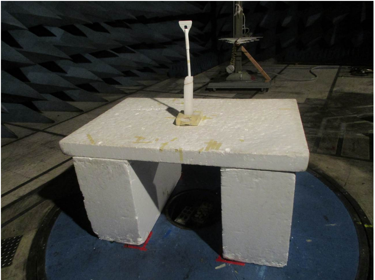
Figure 4: Radiated Emissions – Back View – 200 MHz – 1 GHz
