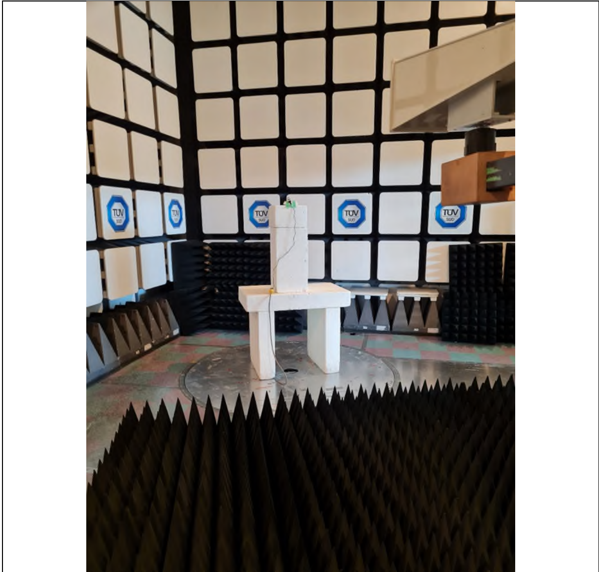
Figure 5 – Radiated Emissions Setup 6GHz to 12GHz Spurious Scans & Band-Edge Measurements
