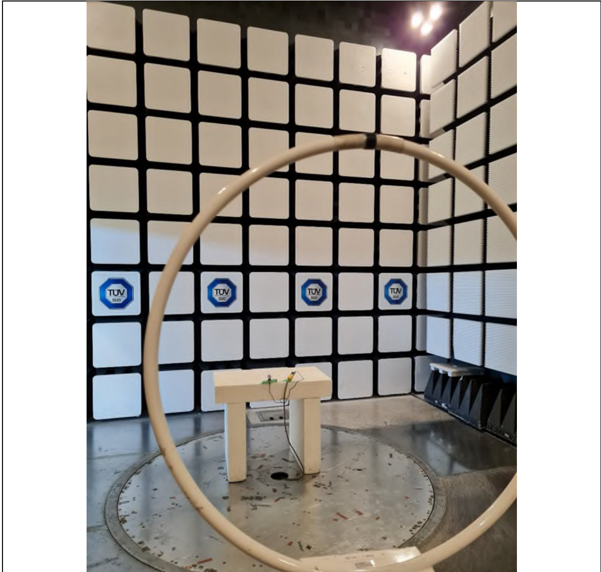
Figure 2 – Radiated Emissions Setup 9kHz to 30MHz
