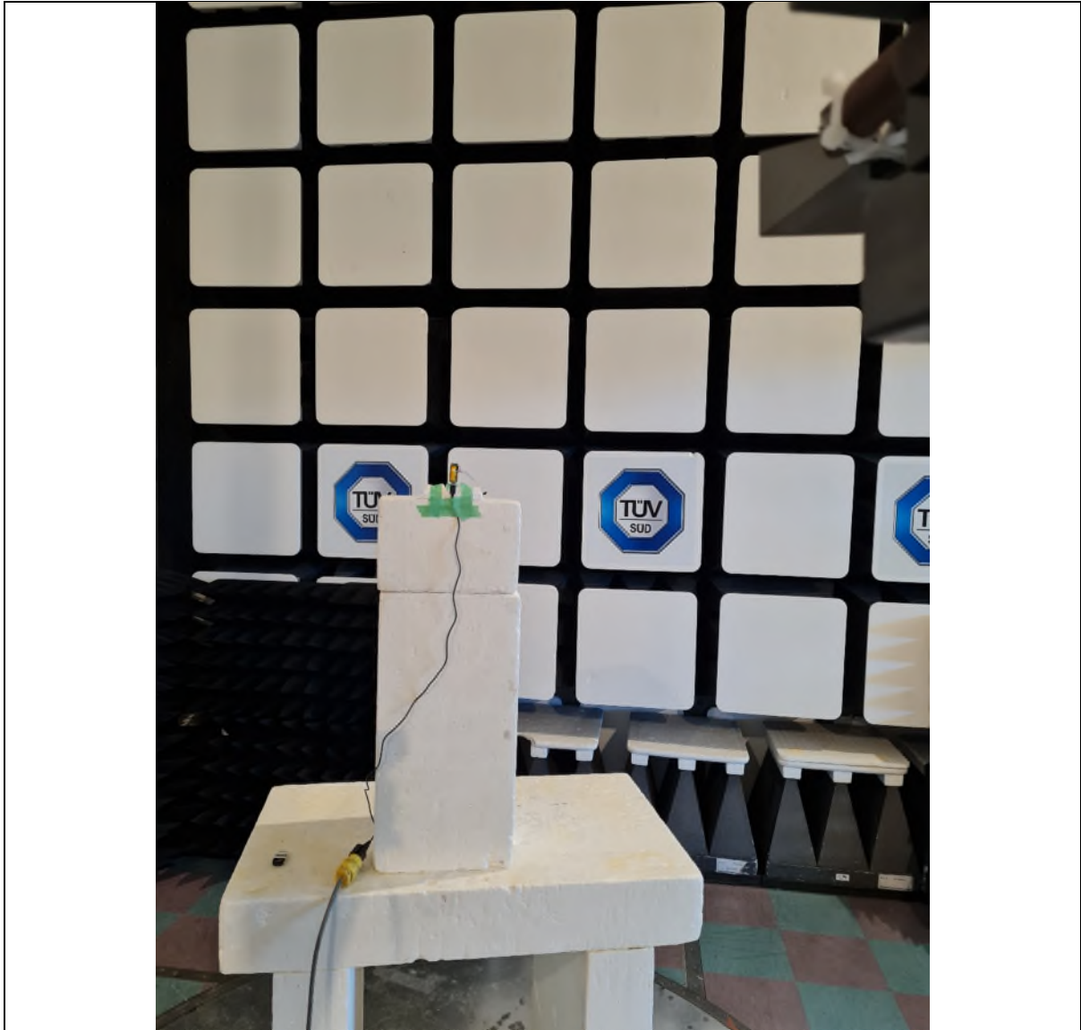
Figure 6 – Radiated Emissions Setup 18GHz to 26GHz Spurious Scans
