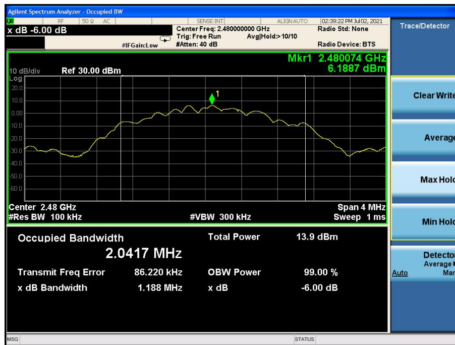
Fig.18 6dB Bandwidth: 2M Ch39
