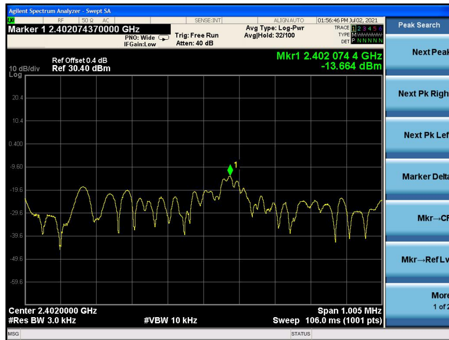
Fig.7 Power spectral density: 2M CH0 PSD/3KHz
