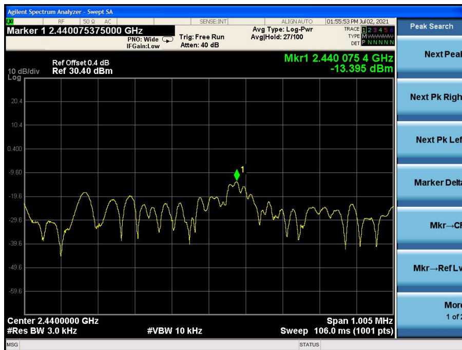
Fig.8 Power spectral density: 2M CH19 PSD/3KHz
