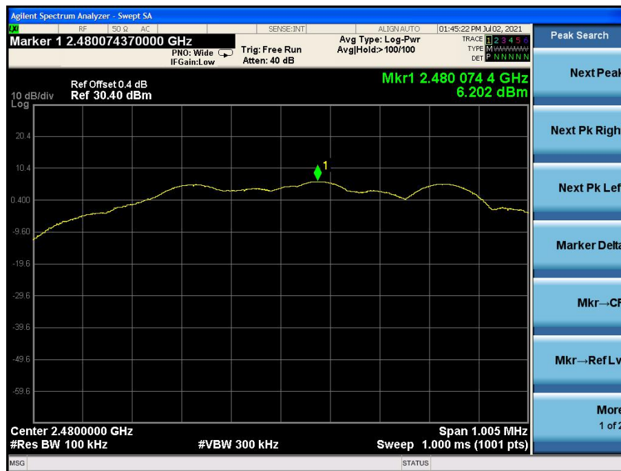
Fig.6 Power spectral density: 1M CH39 PSD/100KHz
