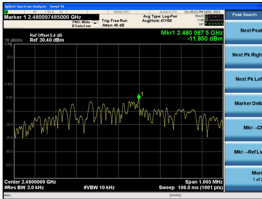
Fig.3 Power spectral density: 1M CH39 PSD/3KHz
