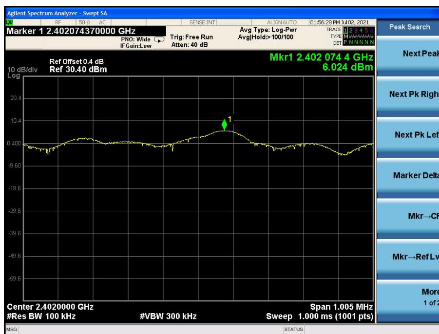
Fig.10 Power spectral density: 2M CH0 PSD/100KHz
