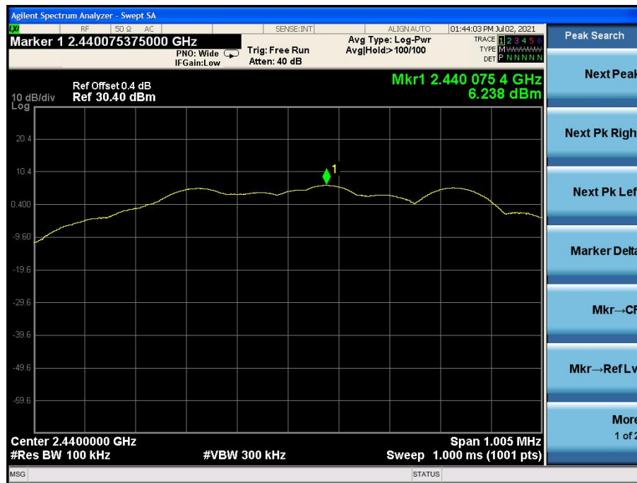
Fig.5 Power spectral density: 1M CH19 PSD/100KHz
