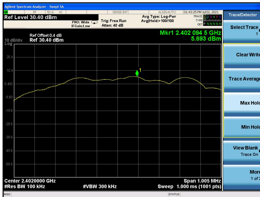
Fig.4 Power spectral density: 1M CH0 PSD/100KHz
