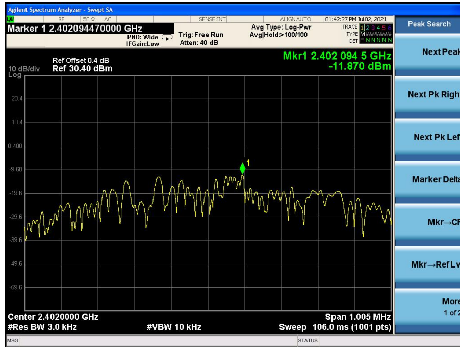
Fig.1 Power spectral density: 1M CH0 PSD/3KHz
