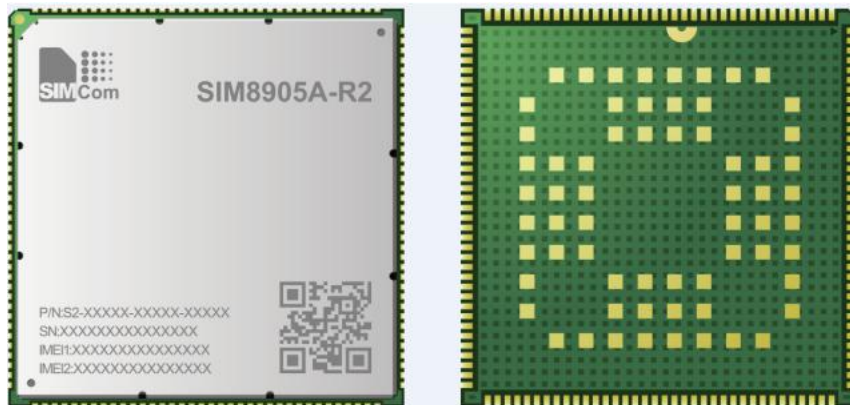
Figure 1: Top and Bottom view of SIM8905A-R2
