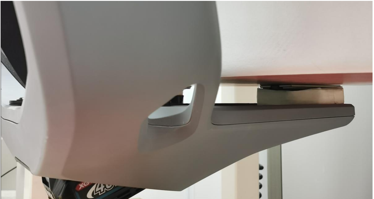
Figure 8 The DUT under the phantom with 0mm separation distance, the side against the user, test position.
