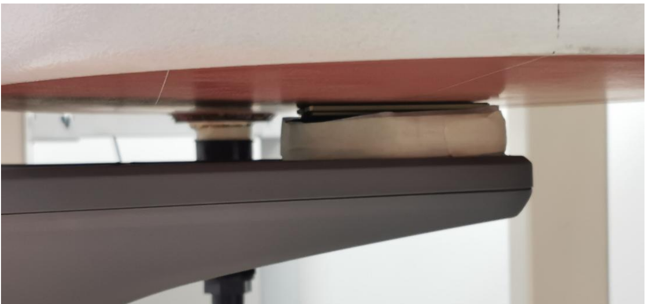
Figure 9 The DUT under the phantom with 0mm separation
