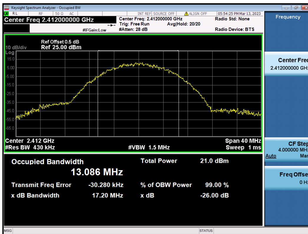
Figure 2: The plots of 99% Bandwidth, 802.11b, 2412MHz
