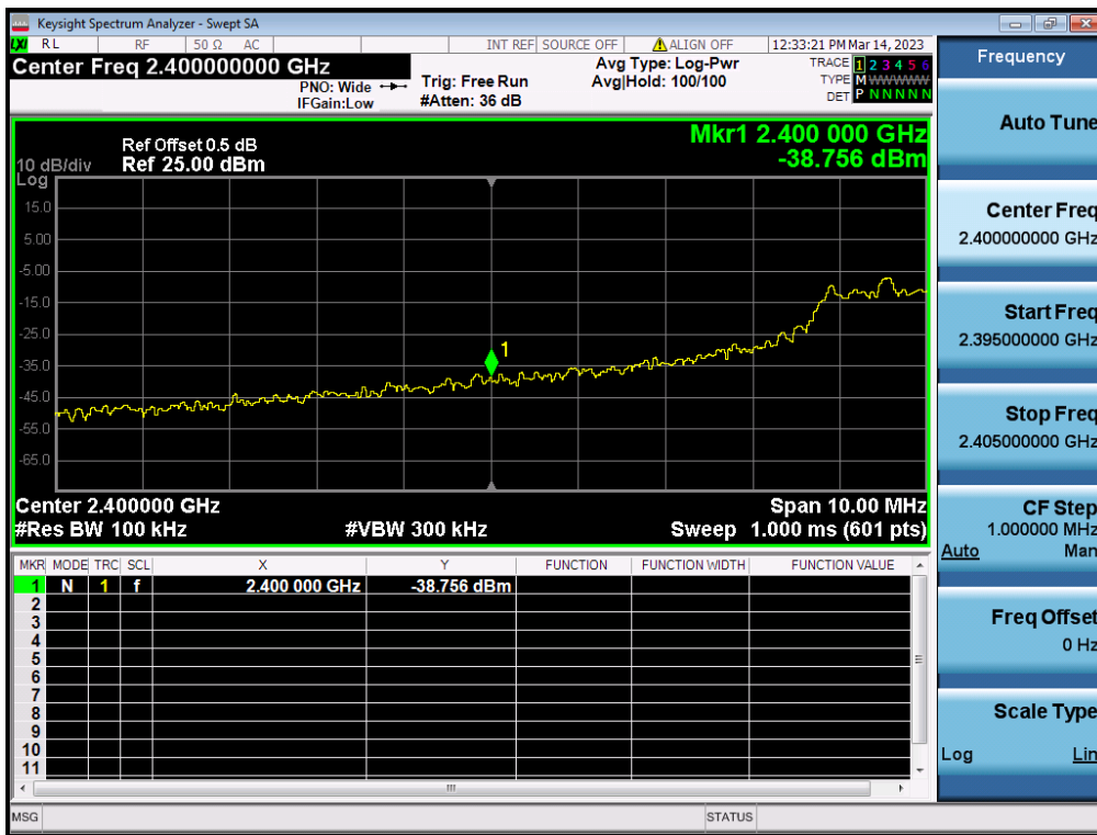
Figure 72: The plots of Conducted Spurious Emission & Authorized-band band-edge, 802.11n(HT40), 2422MHz Conducted spurious emissions 30MHz-3GHz
