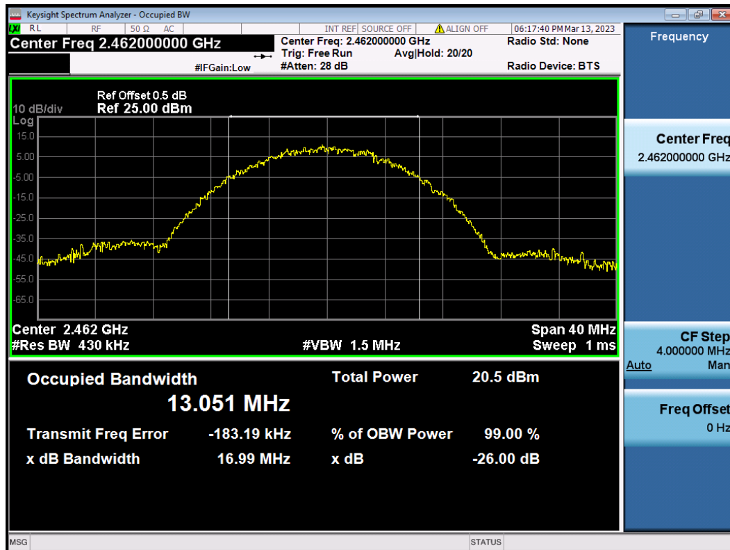
Figure 6: The plots of 99% Bandwidth, 802.11b, 2462MHz
