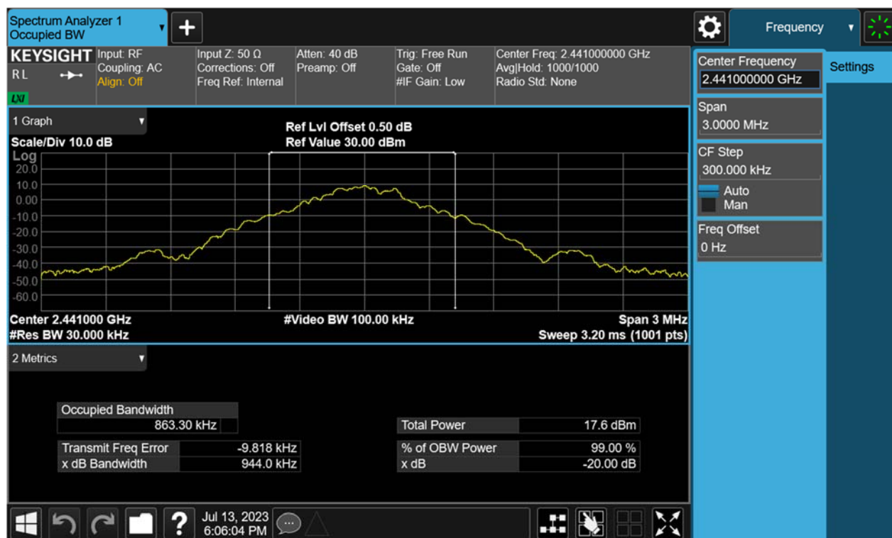
Figure 11: 20dB Bandwidth, 2441MHz, GFSK
