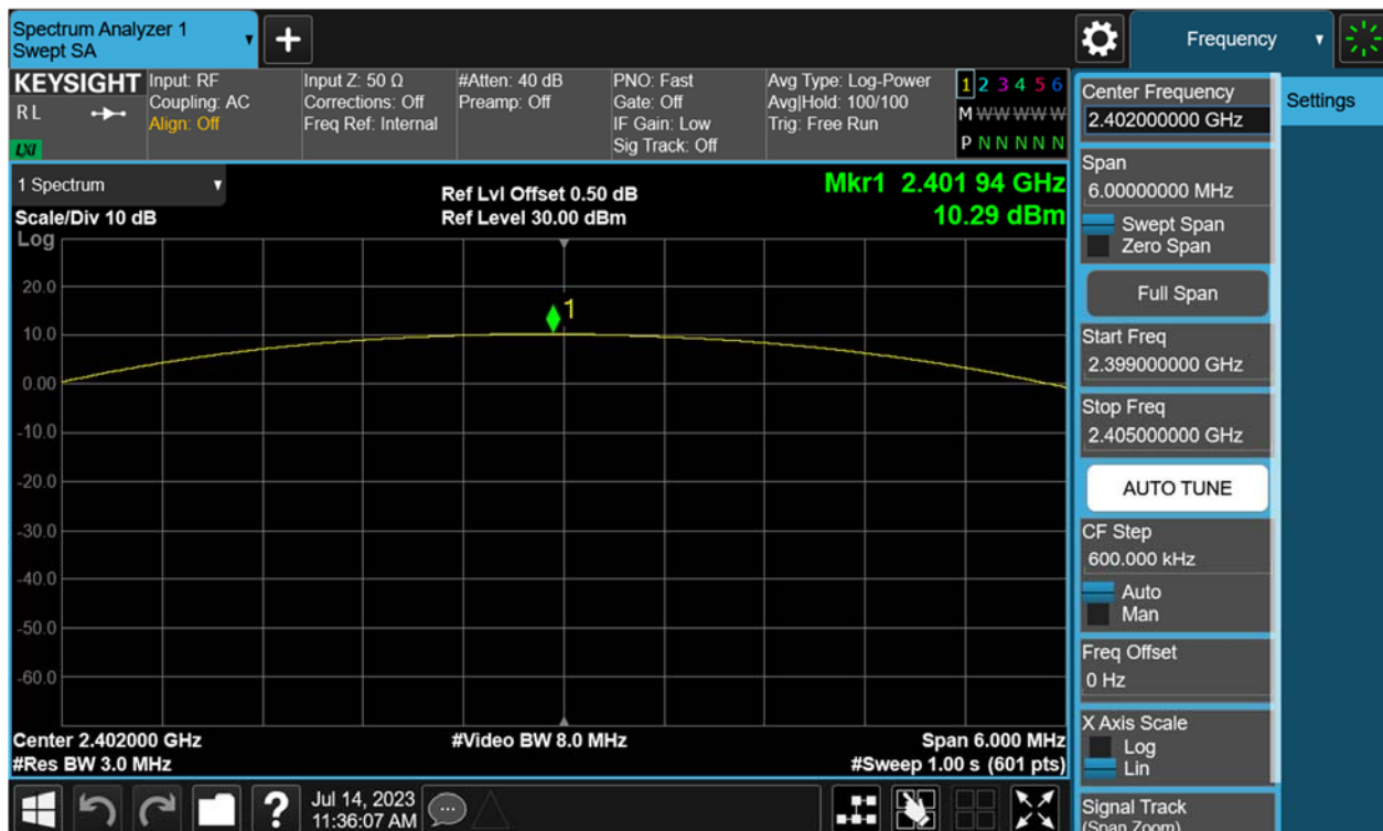
Figure 8: Maximum Peak Output Power, 2441MHz, 8-DPSK
