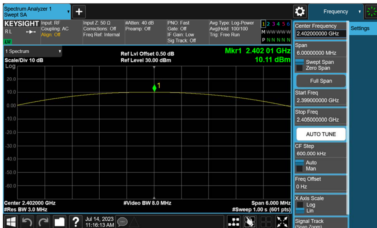
Figure 4: Maximum Peak Output Power, 2402MHz, \pi/4 -DQPSK
