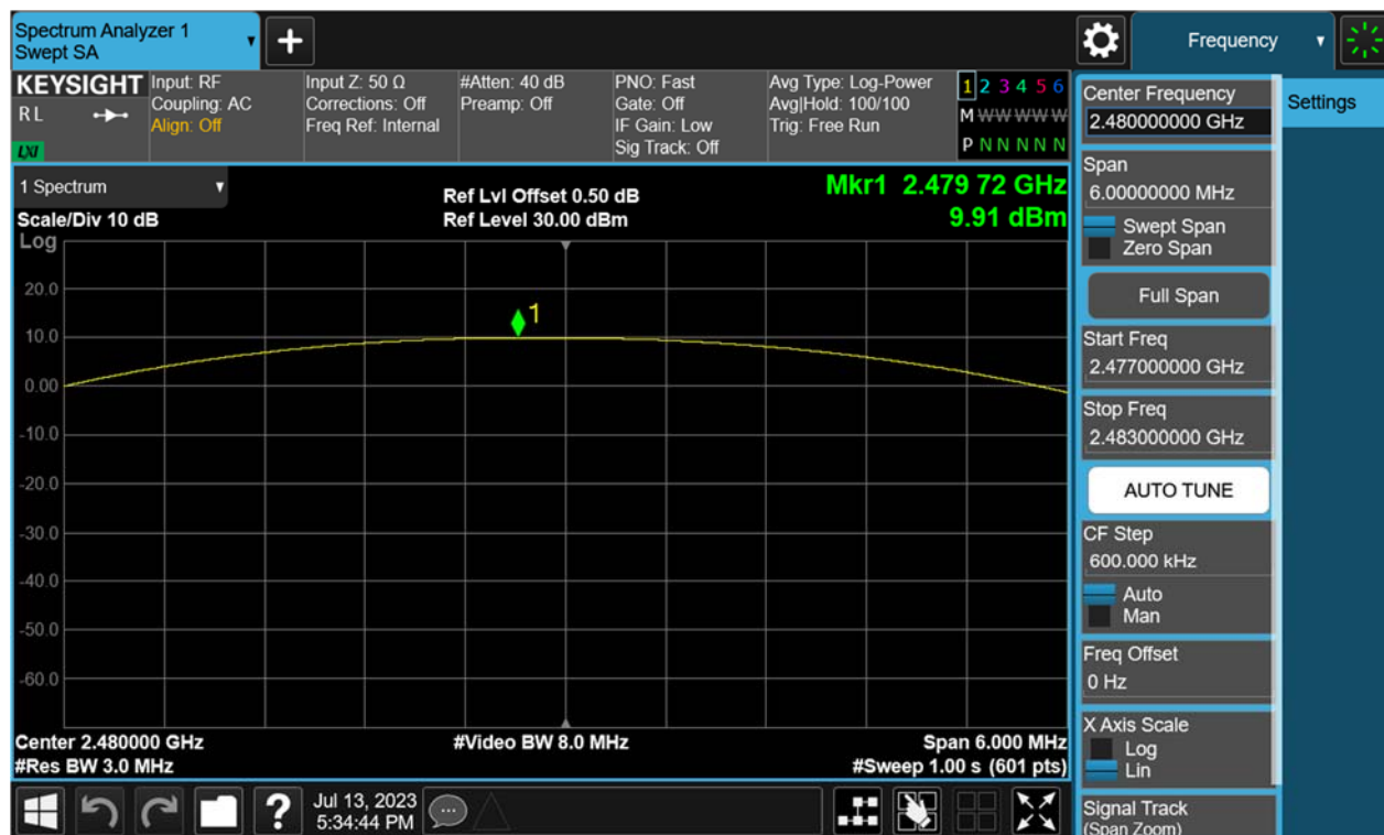
Figure 4: Maximum Peak Output Power, 2402MHz, \pi/4 -DQPSK
