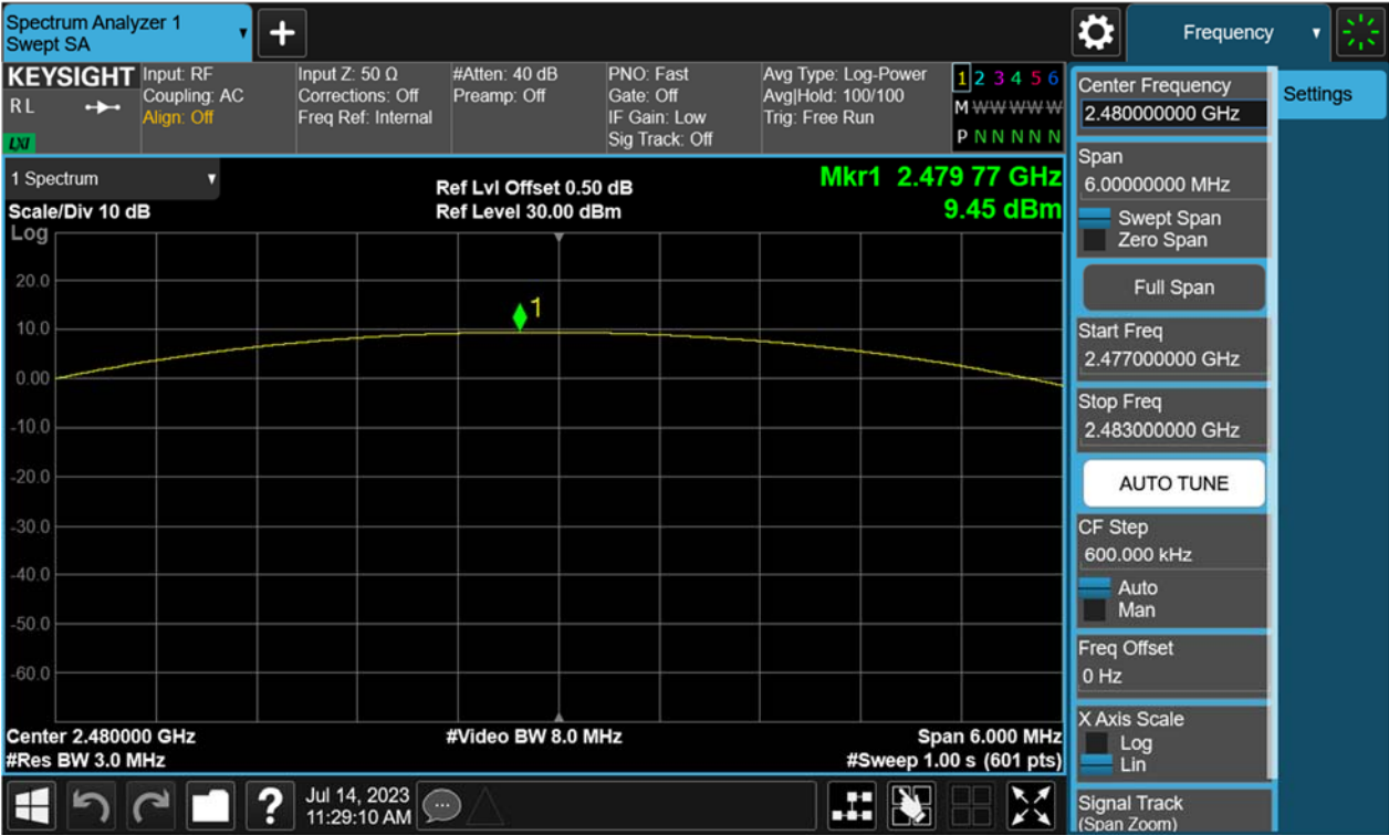
Figure 6: Maximum Peak Output Power, 2480MHz, \pi/4 -DQPSK
