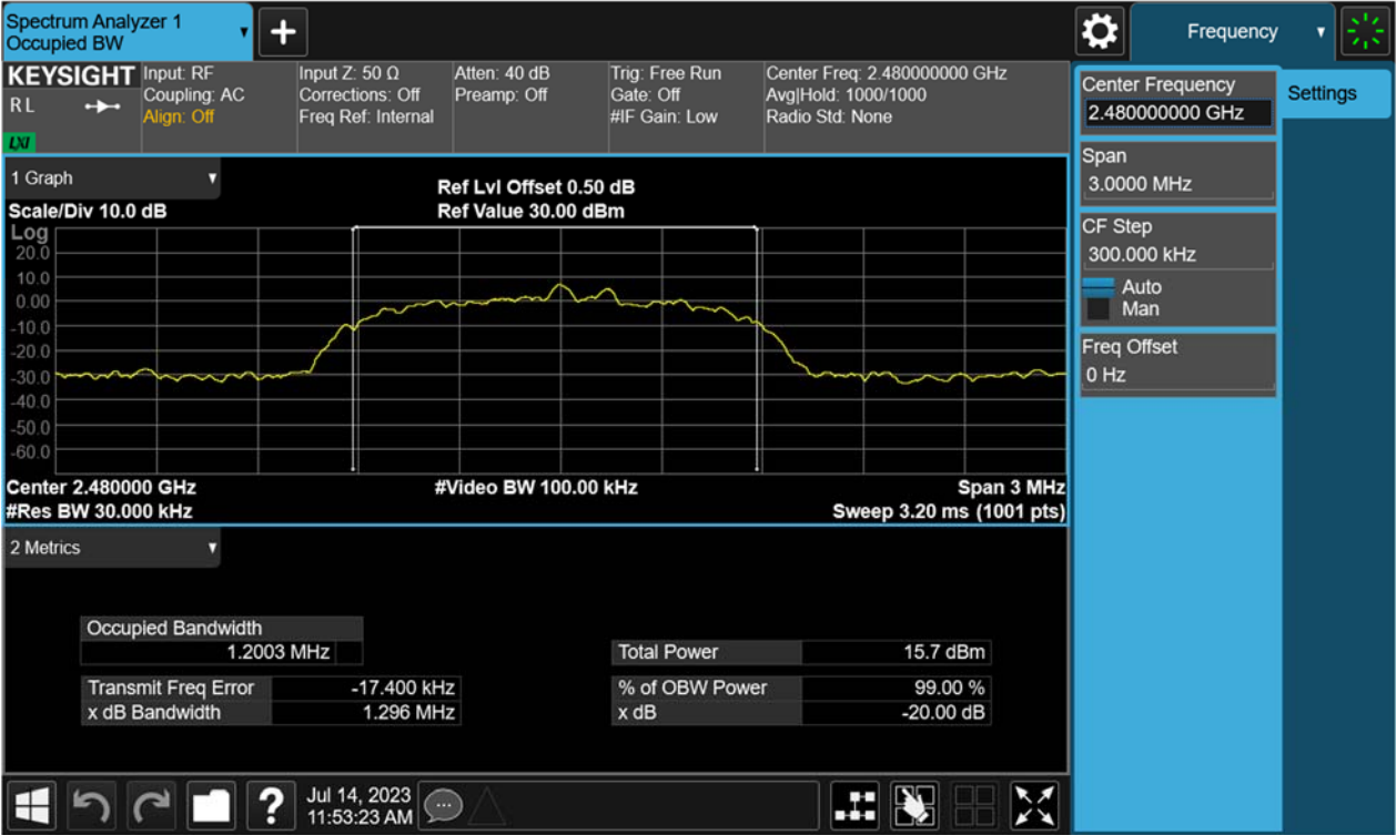
Figure 18: 20dB Bandwidth, 2480MHz, 8-DPSK
