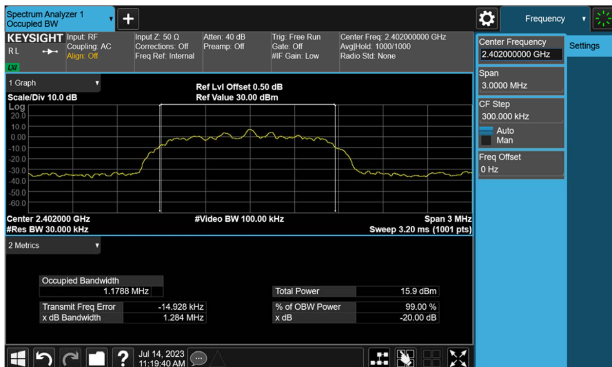
Figure 13: 20dB Bandwidth, 2402MHz, \pi/4 -DQPSK
