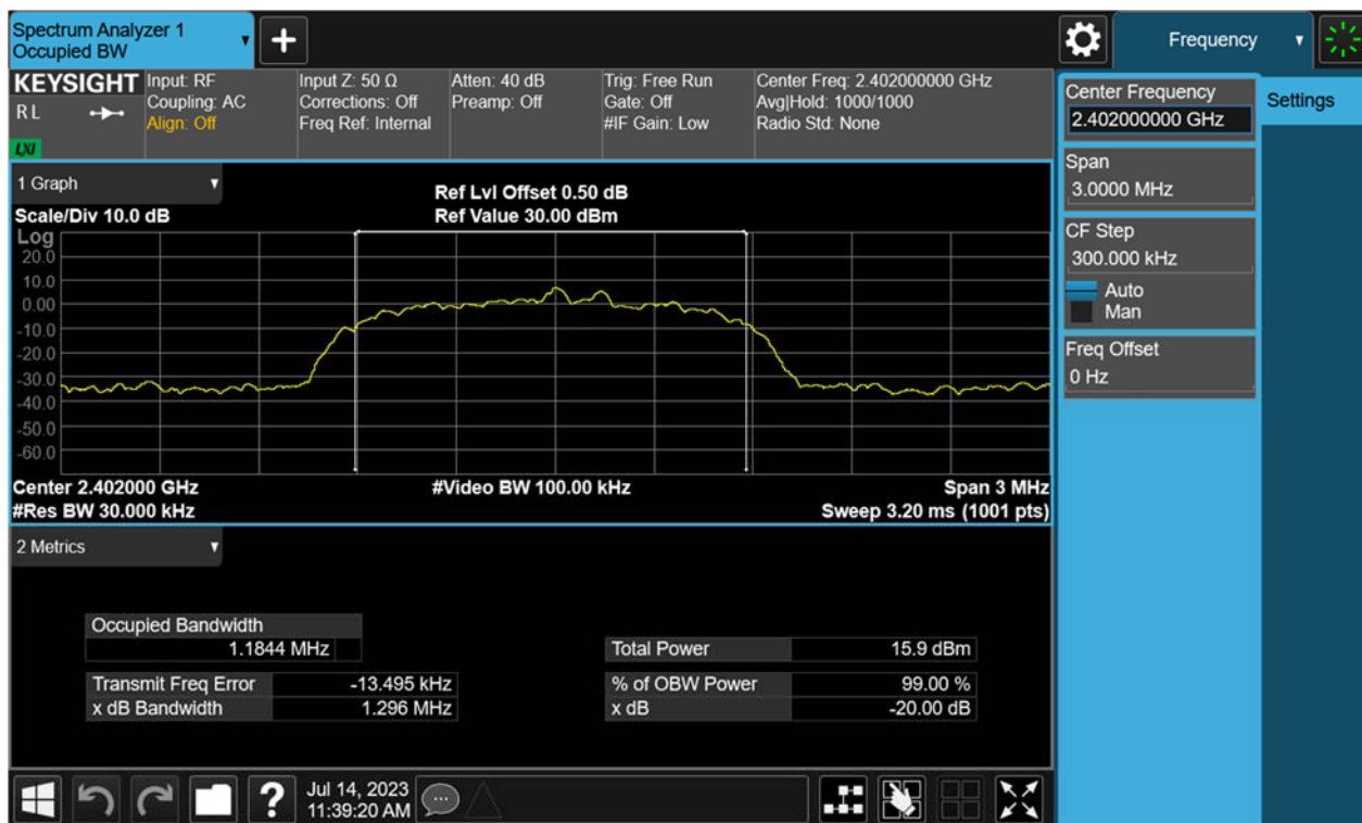
Figure 17: 20dB Bandwidth, 2441MHz, 8-DPSK
