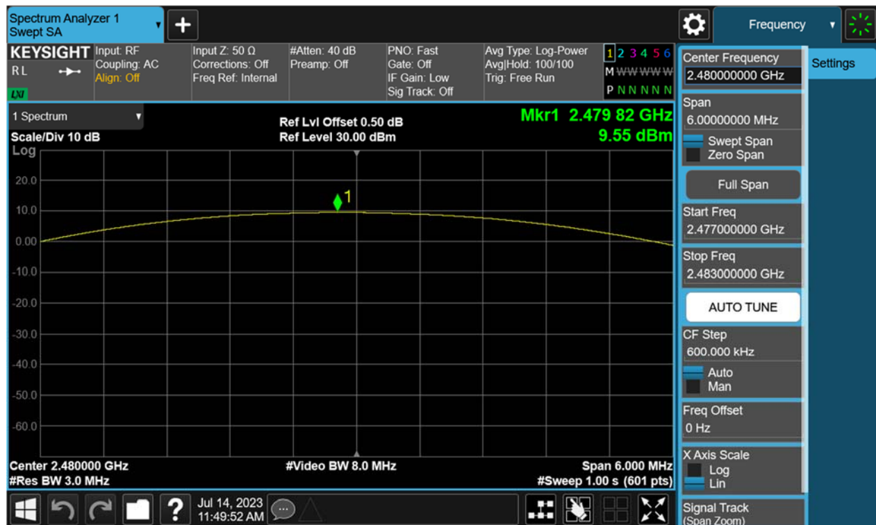
Figure 9: Maximum Peak Output Power, 2480MHz, 8-DPSK
