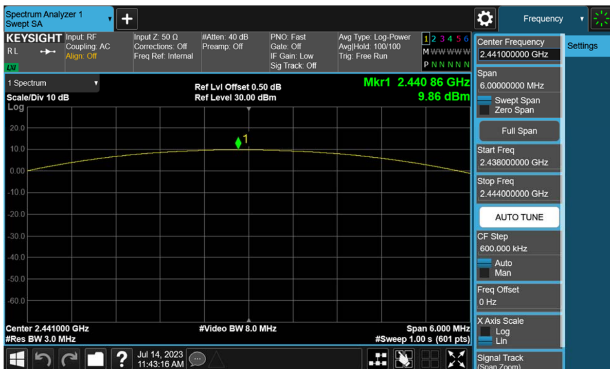
Figure 8: Maximum Peak Output Power, 2441MHz, 8-DPSK
