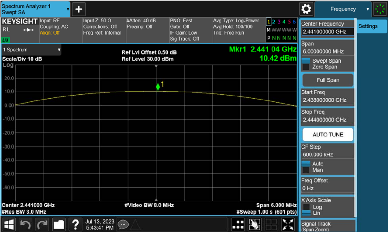
Figure 2: Maximum Peak Output Power, 2441MHz, GFSK
