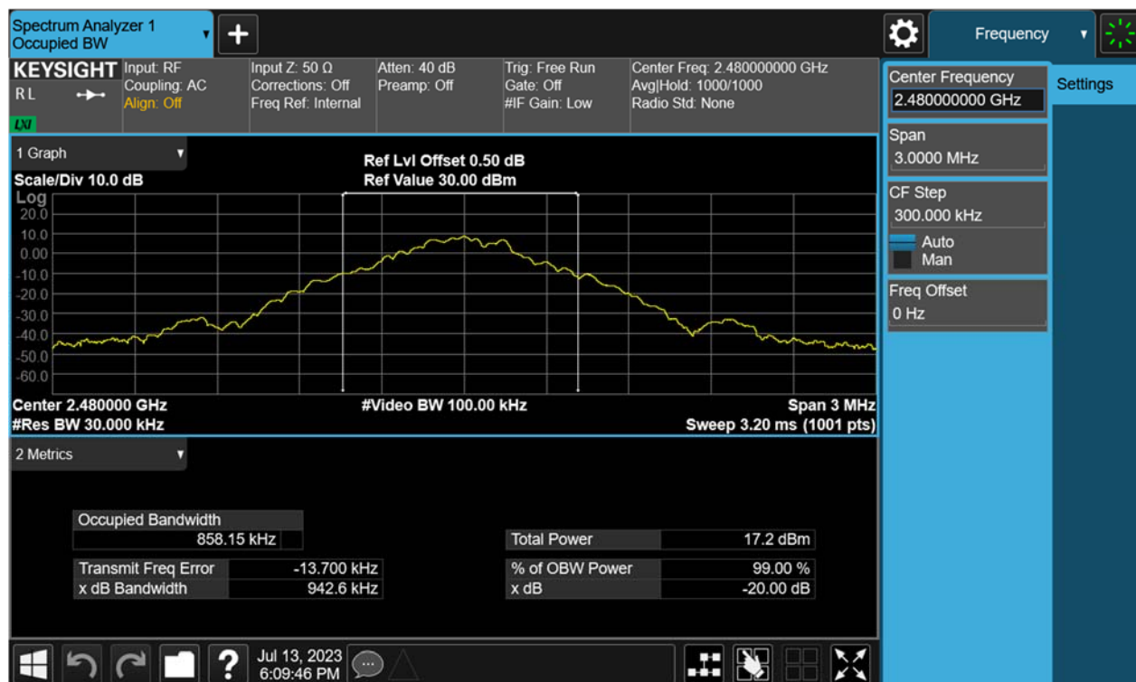
Figure 13: 20dB Bandwidth, 2402MHz, \pi/4 -DQPSK
