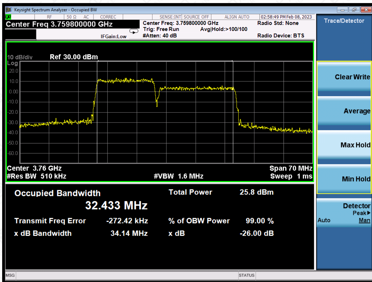
LTE CA band 43Part27 , 15MHz+20MHz Bandwidth,16QAM (99% BW)
