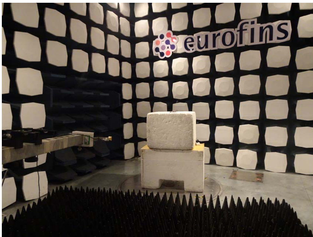
Picture 1: Radiated Spurious Emissions Test setup
