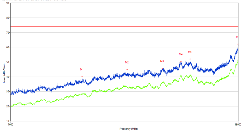
REmission Test case_FCC_Part 15C_FCC 15.249_7GHz-18GHz
