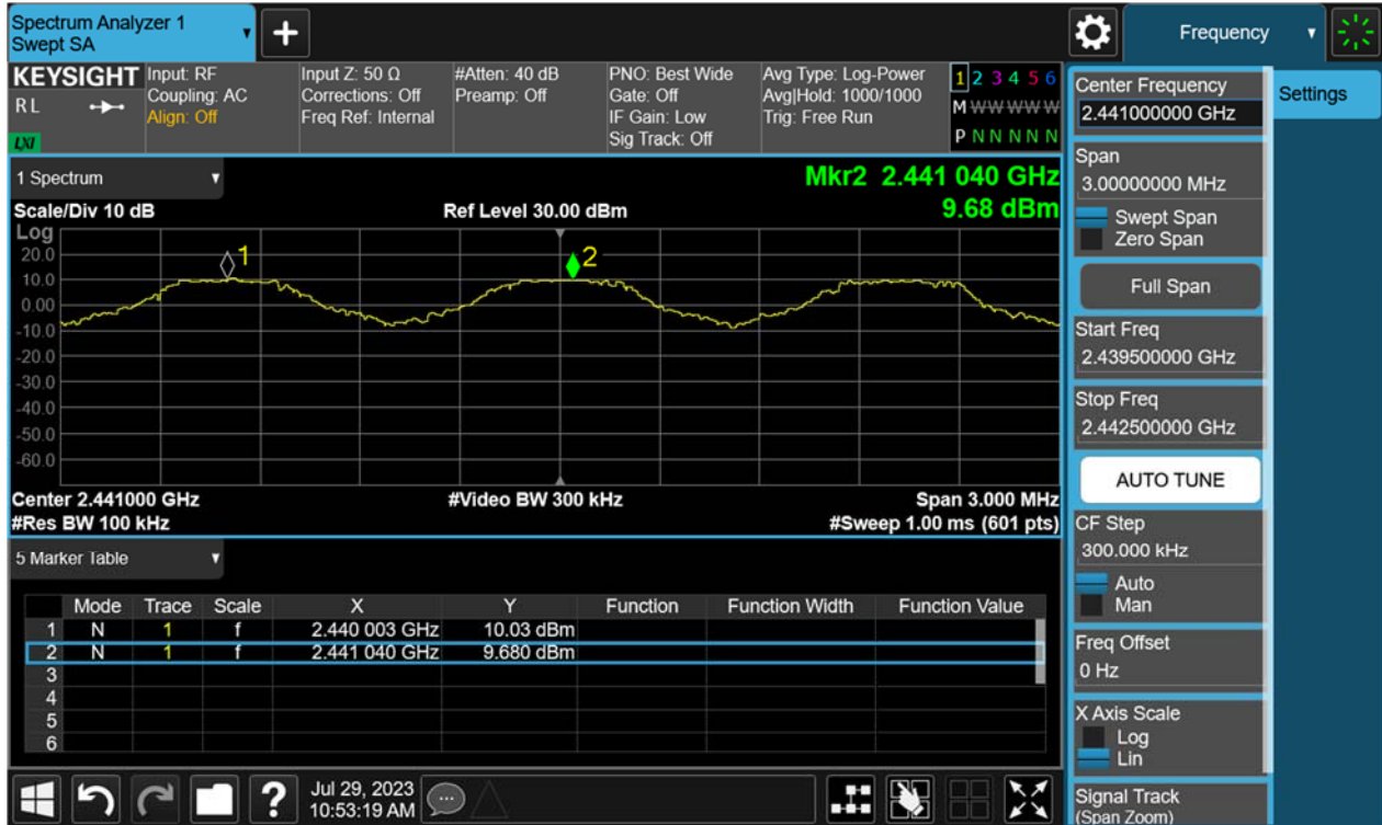
Figure 32: Hopping Frequency Separation, Hopping Mode, \pi/4 -DQPSK
