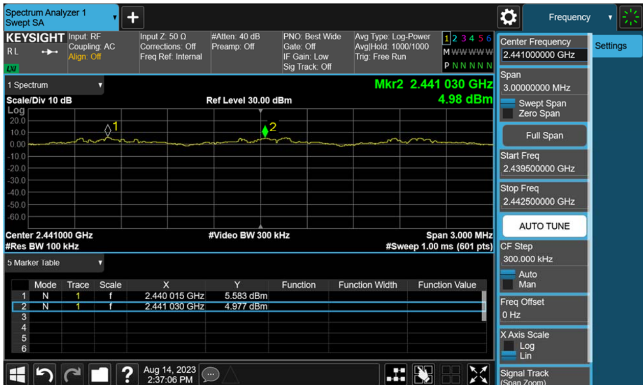
Figure 32: Hopping Frequency Separation, Hopping Mode, \pi/4 -DQPSK
