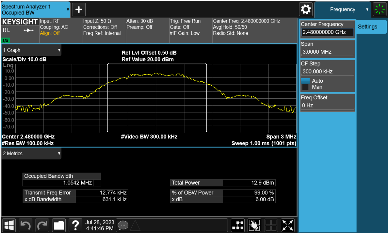
Figure 6: 6dB Bandwidth, 2480MHz
