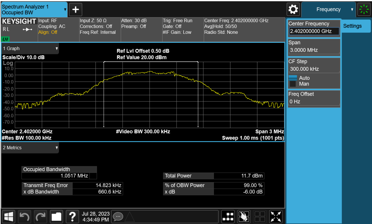
Figure 4: 6dB Bandwidth, 2402MHz
