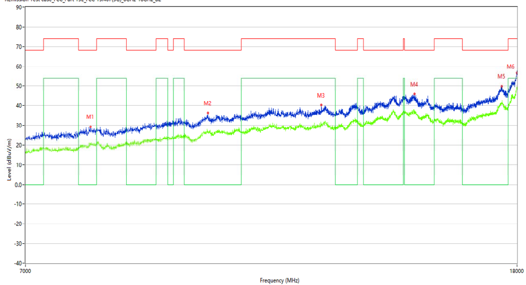
R Emission Test case_FCC_Part 15E_FCC 15.407(5G)_6GHz-18GHz_B2
