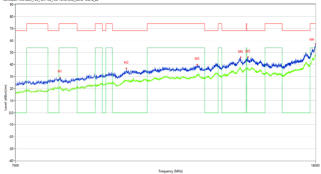
R Emission Test case_FCC_Part 15E_FCC 15.407(5G)_6GHz-18GHz_B2
