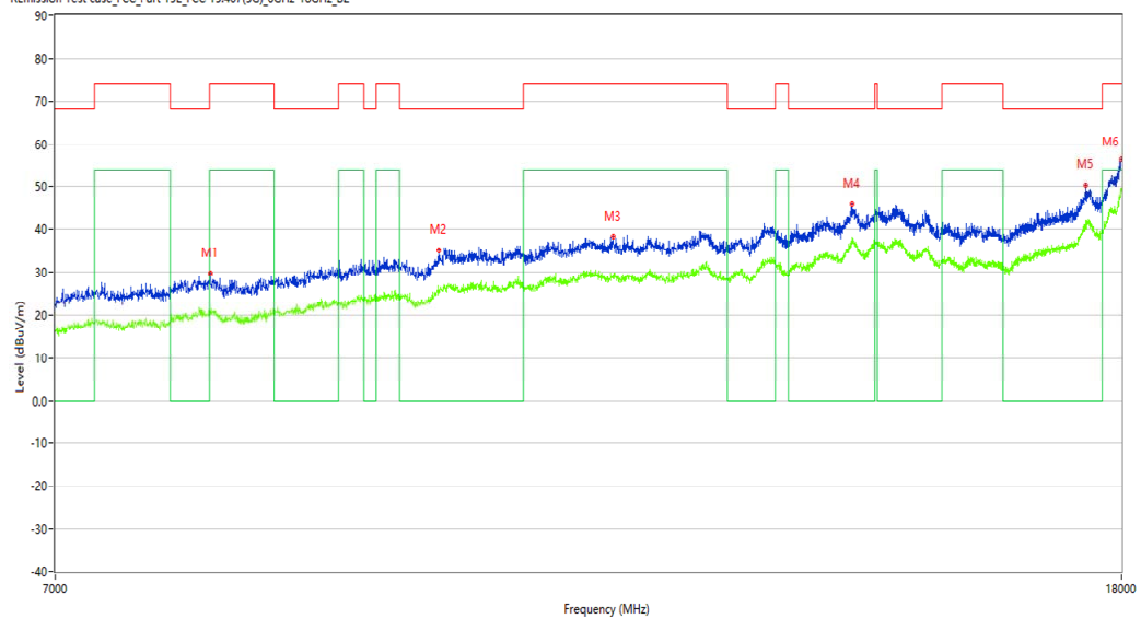
R Emission Test case_FCC_Part 15E_FCC 15.407(5G)_6GHz-18GHz_B2
