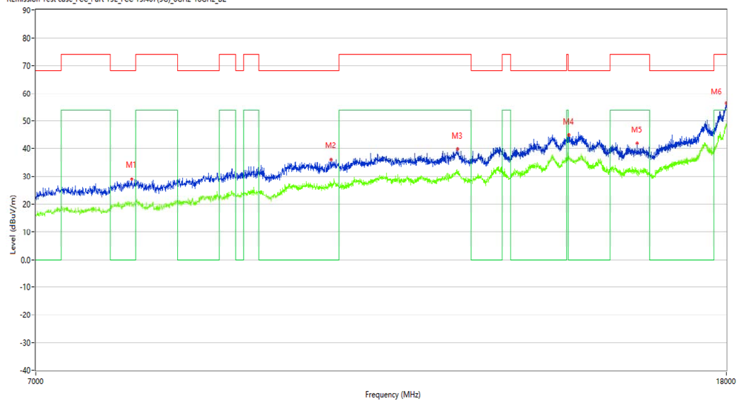
R Emission Test case_FCC_Part 15E_FCC 15.407(5G)_6GHz-18GHz_B2
