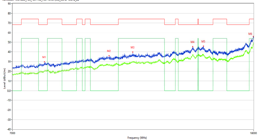
R Emission Test case_FCC_Part 15E_FCC 15.407(5G)_6GHz-18GHz_B2
