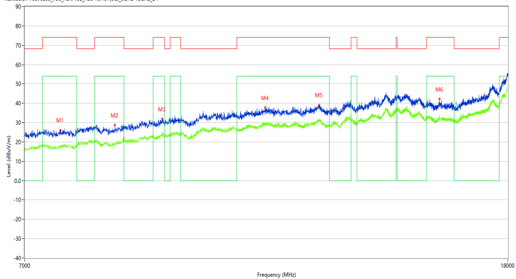
R Emission Test case_FCC_Part 15E_FCC 15.407(5G)_6GHz-18GHz_B1
