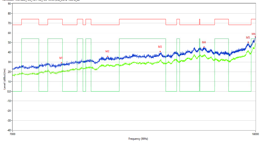
R Emission Test case_FCC_Part 15E_FCC 15.407(5G)_6GHz-18GHz_B2
