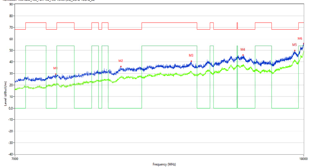
R Emission Test case_FCC_Part 15E_FCC 15.407(5G)_6GHz-18GHz_B2
