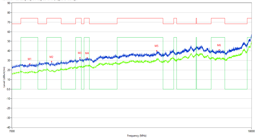
R emission Test case_FCC_Part 15E_FCC 15.407(5G)_6GHz-18GHz_B1
