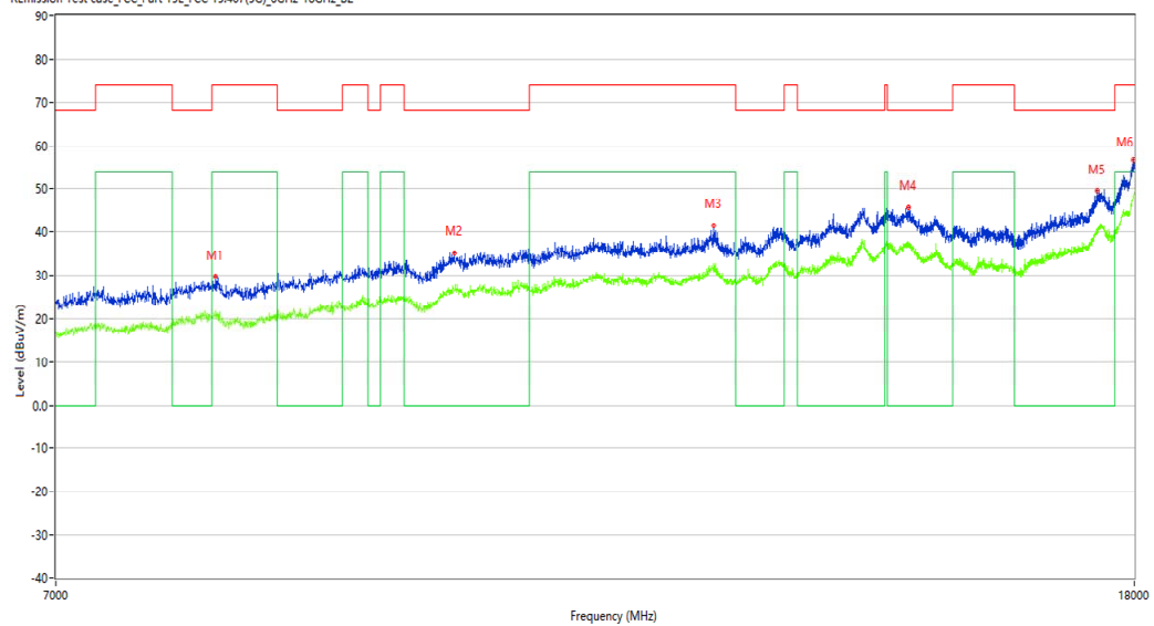
R Emission Test case_FCC_Part 15E_FCC 15.407(5G)_6GHz-18GHz_B2
