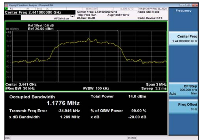
20dB Bandwidth: 8DPSK,2441MHz,3DH5
