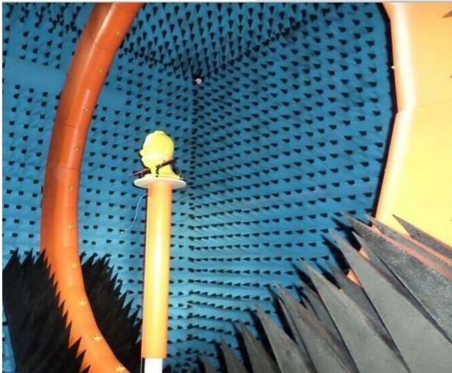
Figure 4.2.1 3D anechoic chamber test coordinate system (back view)
