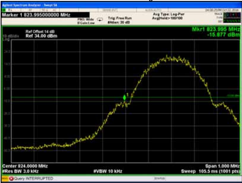
GPRS 850 band edge-left side
