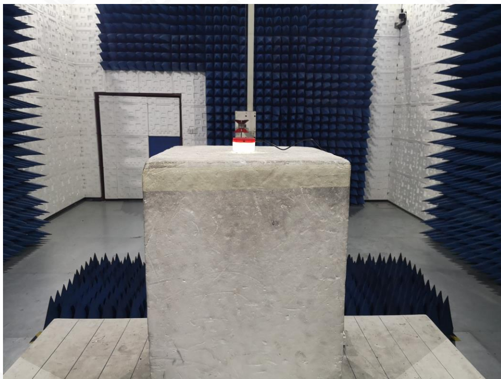
RADIATED EMISSION TEST SETUP ABOVE 1GHZ
