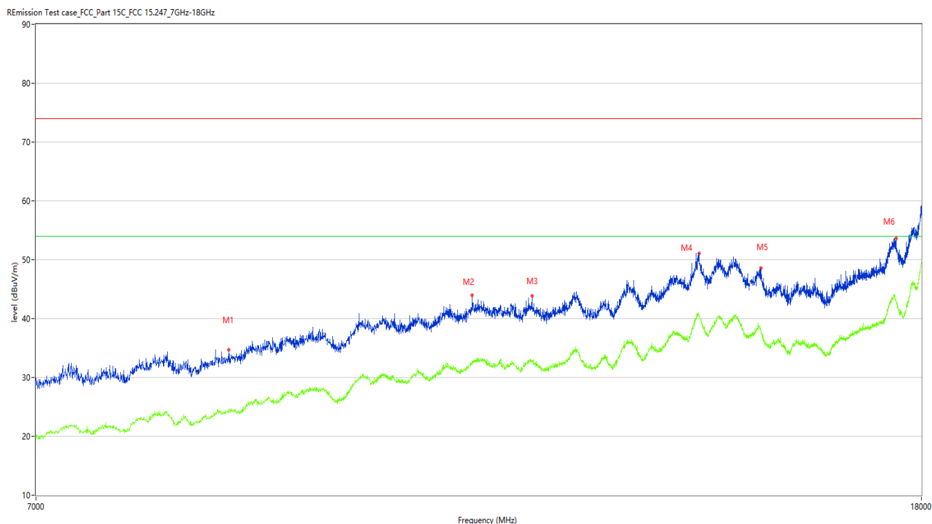
Figure 29: The plots of Radiated Emission, 2403MHz,7GHz-18GHz, Vertical polarization
