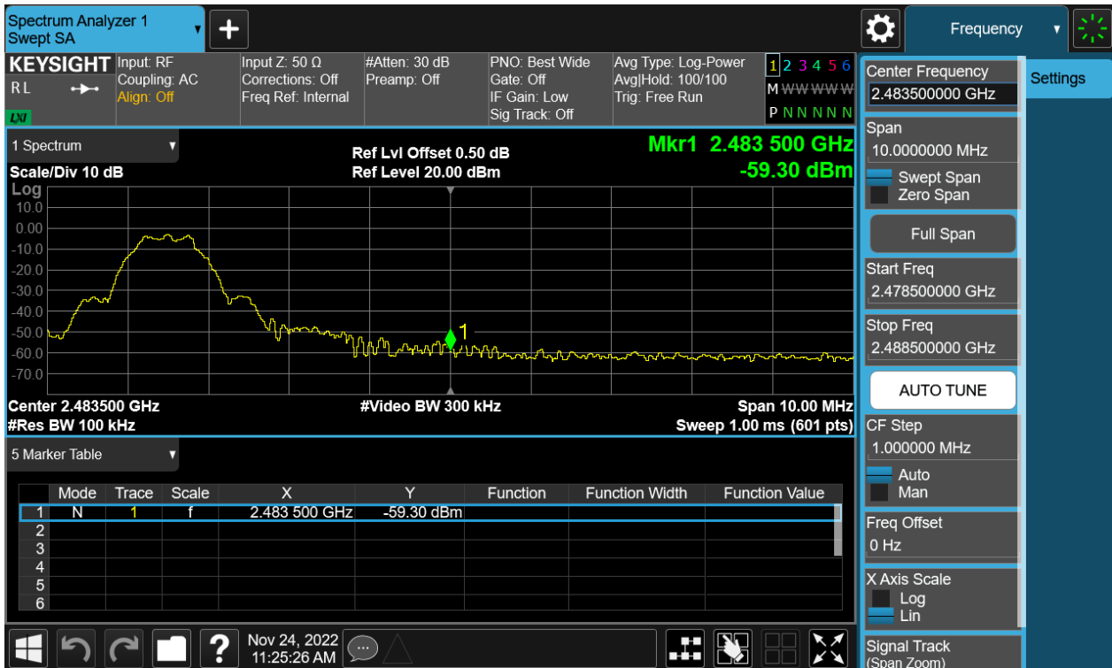
Figure 22: The plots of Conducted Spurious Emission & Authorized-band band-edge, 2480MHz, Conducted spurious emissions 30MHz-3GHz
