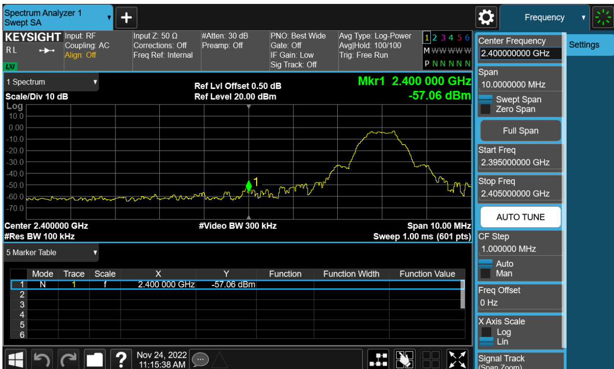
Figure 14: The plots of Conducted Spurious Emission & Authorized-band band-edge, 2403MHz, Band Edge
