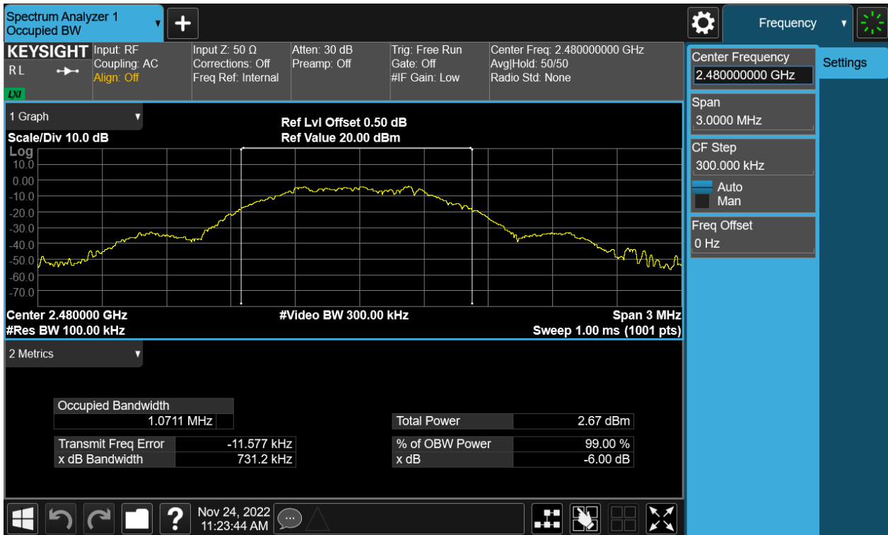
Figure 9: The plots of 99% Bandwidth, 2480MHz
