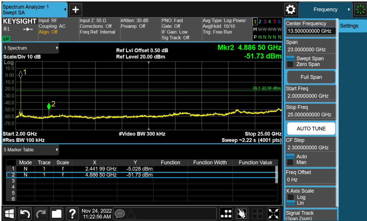
Figure 20: The plots of Conducted Spurious Emission & Authorized-band band-edge, 2480MHz, Carrier Level
