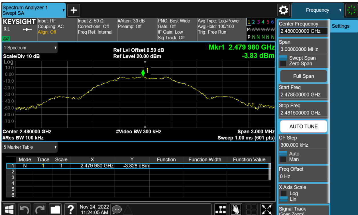
Figure 20: The plots of Conducted Spurious Emission & Authorized-band band-edge, 2480MHz, Carrier Level
