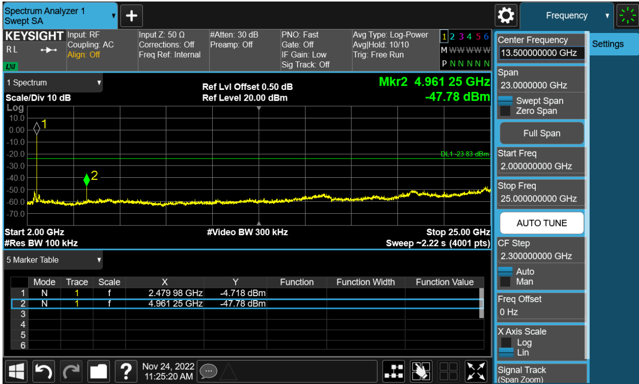
Figure 23: The plots of Conducted Spurious Emission & Authorized-band band-edge, 2480MHz, Conducted spurious emissions 2GMHz-25GHz
