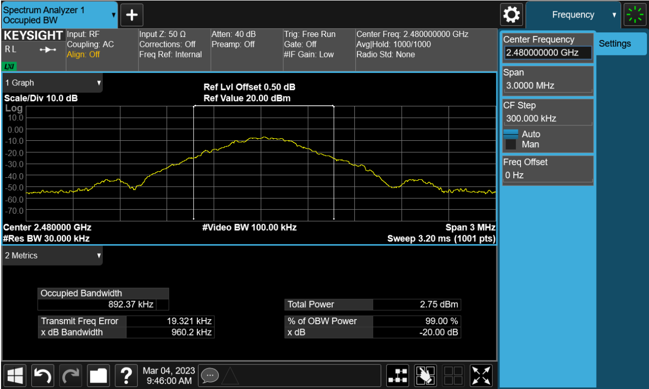
Figure 31: The plots of 20dB Bandwidth and 99% Bandwidth, 2480MHz
