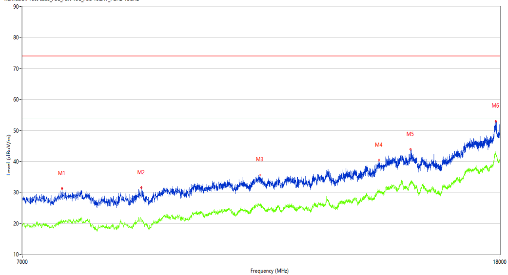
REmission Test case_FCC_Part 15C_FCC 15.247.7GHz-18GHz
