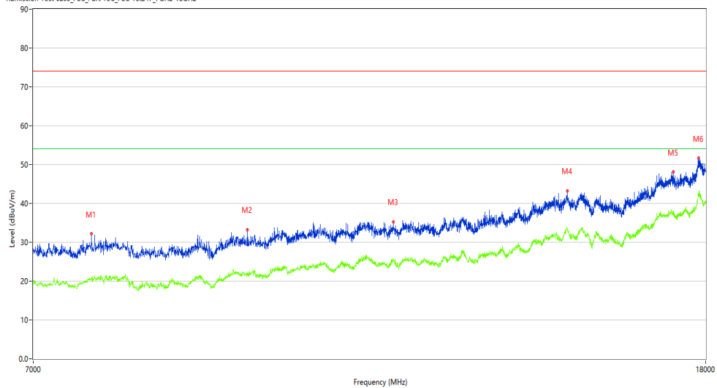
REmission Test case_FCC_Part 15C_FCC 15.247_7GHz-18GHz
