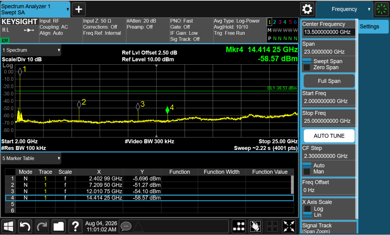
Figure 11: The plots of Conducted Spurious Emission & Authorized-band band-edge, 2442MHz Carrier Level
