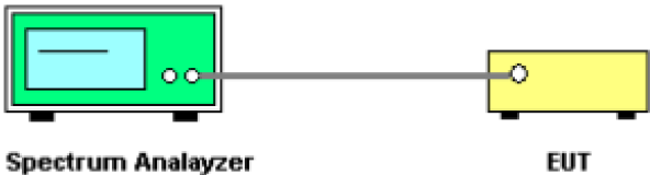
Diagram of Measurement Equipment Configuration for Transmitter Test
