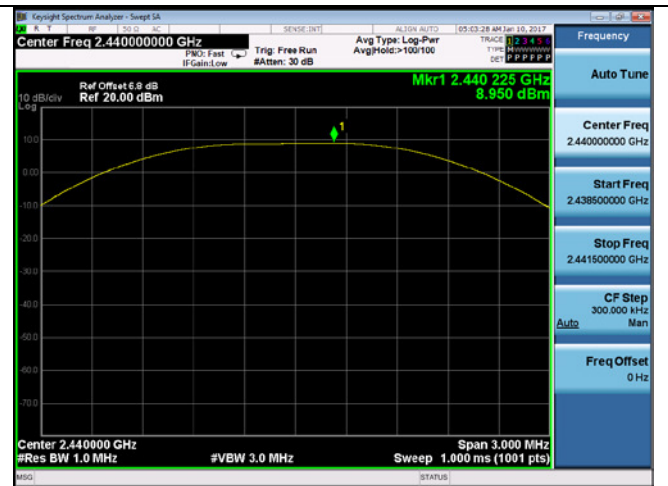
Output Power –Bluetooth LE 2440MHz
