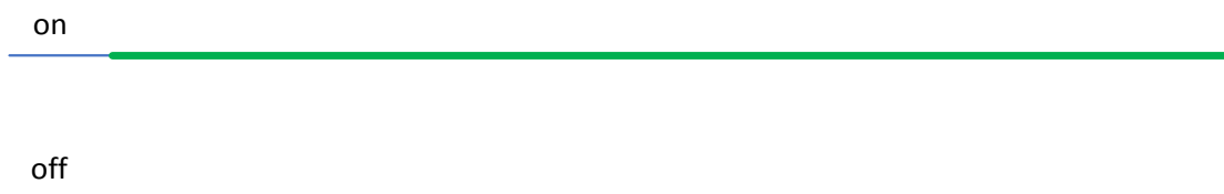
Figure 6: Flashing pattern in status Connected
