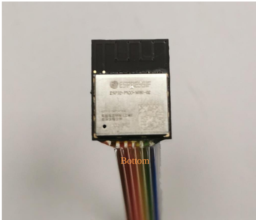
Figure 4 ESP32-PICO-MINI-02 Module attached with wires
