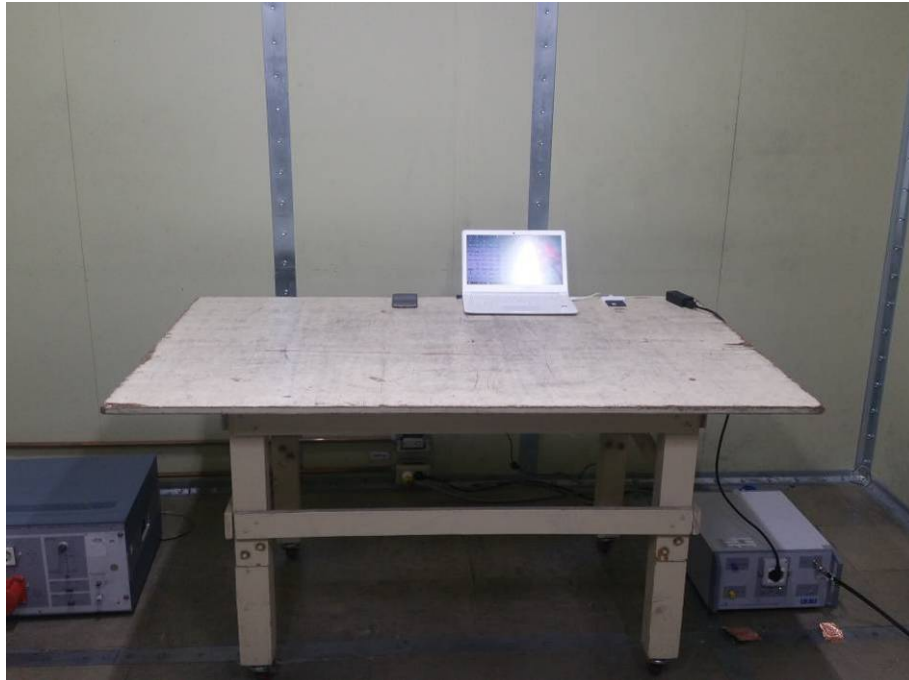
Photograph 4 : Setup for Conducted Emissions
