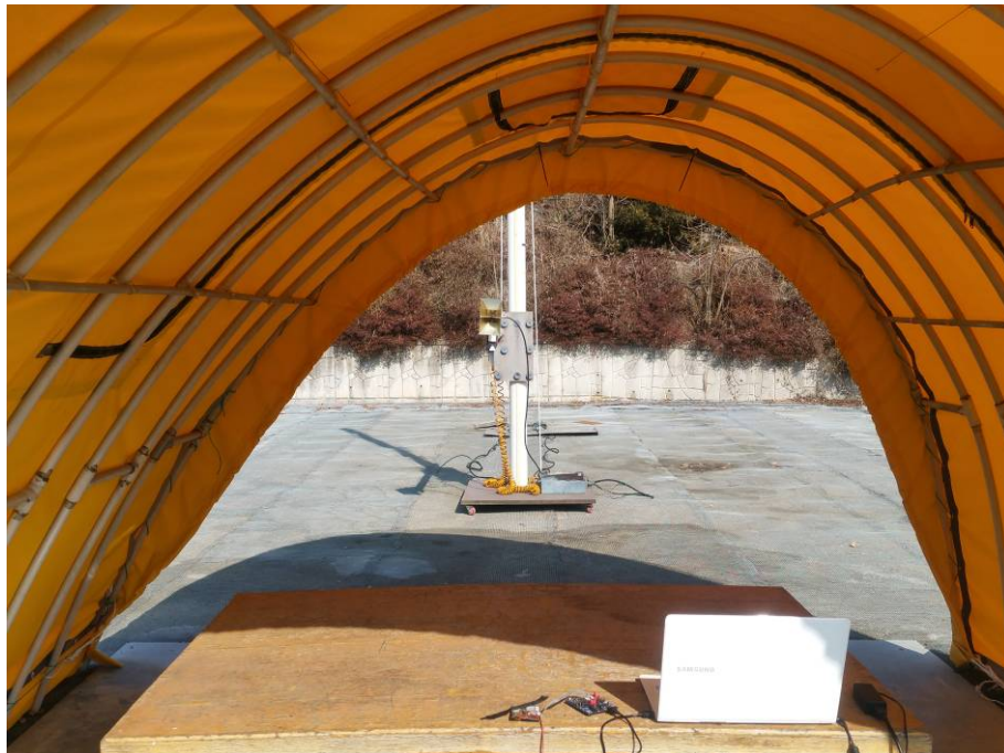
Photograph 3 : Setup for radiated Emissions (above 1 GHz)
