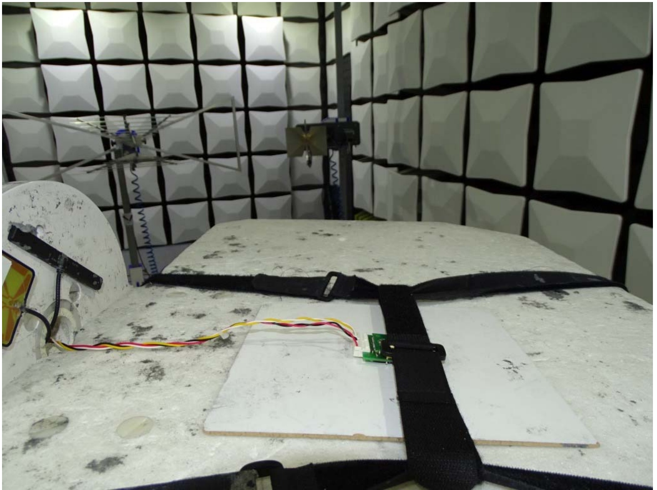
Photo 8: Test setup for radiated measurements above 1 GHz, detailed view EUT fixed on EUT-positioning device, view to horn antenna
