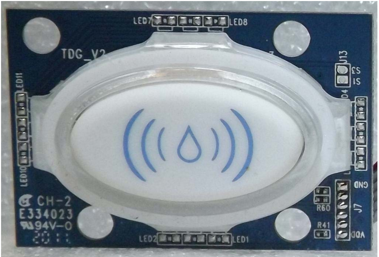
Figure E22.8 – Pushbutton PCB, Component Side
