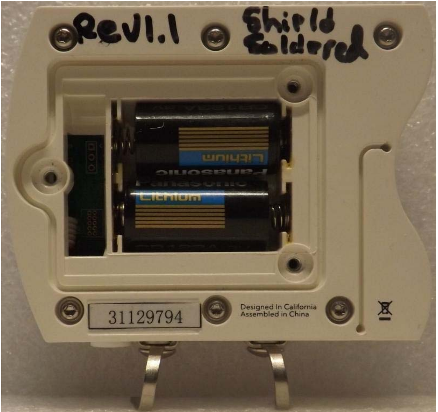
Figure E22.1 – Back, Battery Cover Removed
