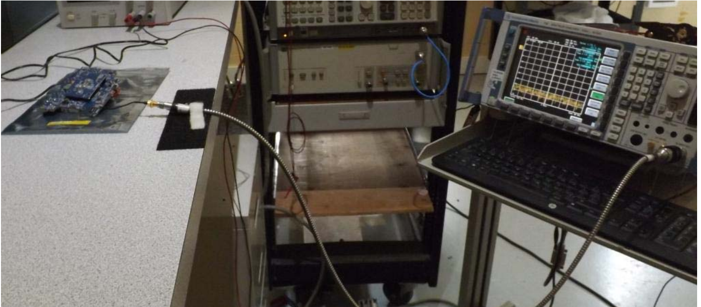
Figure E23.1 – Setup, Antenna Port Conducted Measurements
