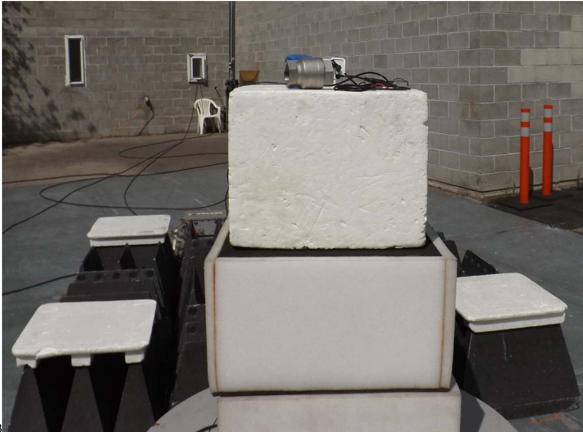
Figure E23.6 – Setup, Radiated Emissions Measurements Above 1000MHz
