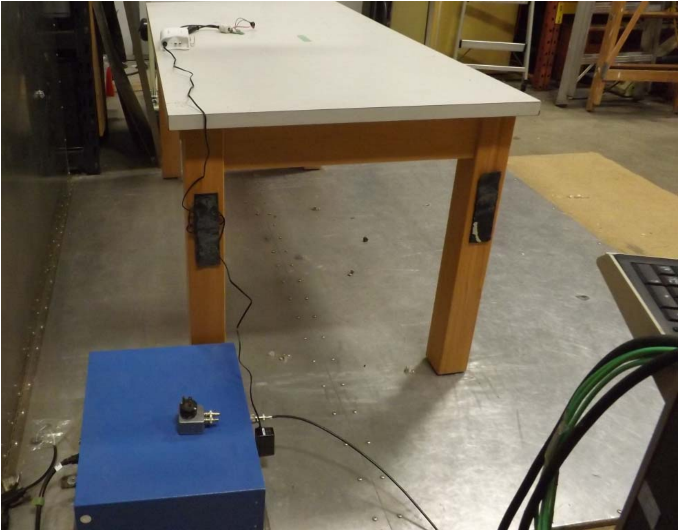
Figure E23.2 – Setup, Line Conducted Measurements
