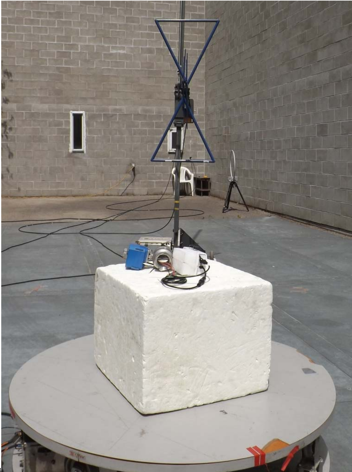
Figure E23.4 – Setup, Radiated Emissions Measurements 30 - 1000MHz
