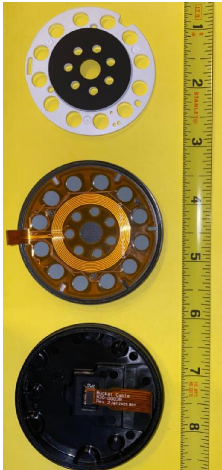
Photograph of Antenna Board and Inside Cover
