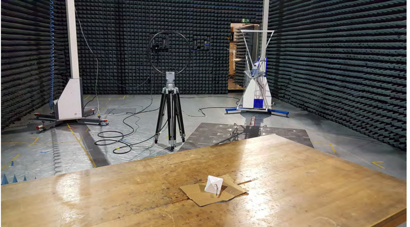
Photo 2: Test setup for radiated measurements (Enclosure, fully-anechoic chamber, 1-18 GHz intentional radiator §15 / 30 MHz – 10/20 GHz §22/24/27)
