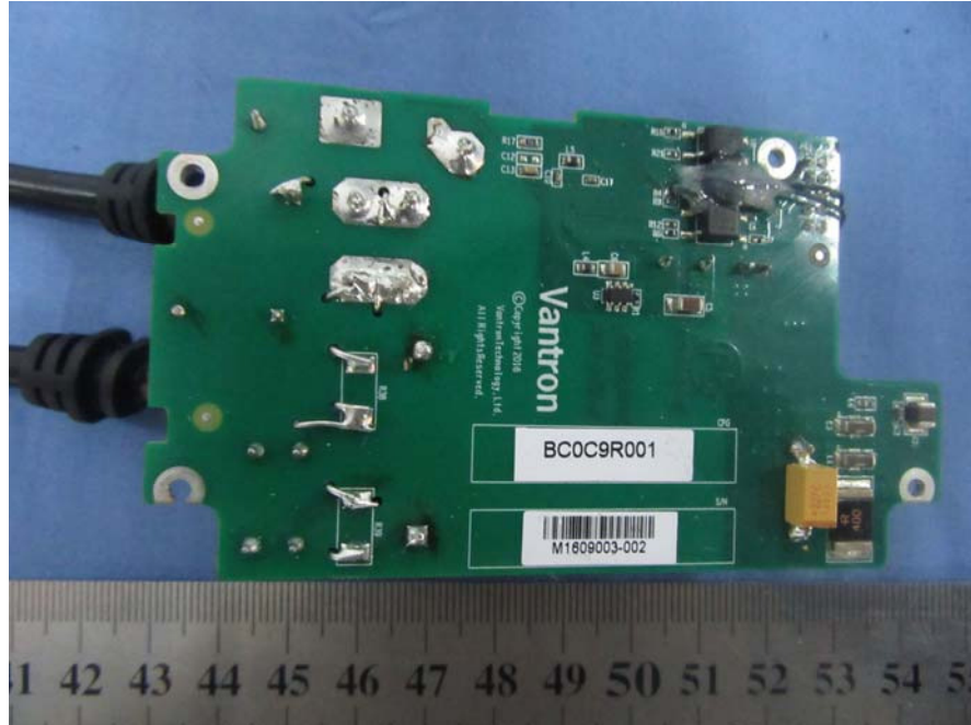
EUT – Power Board Bottom View
