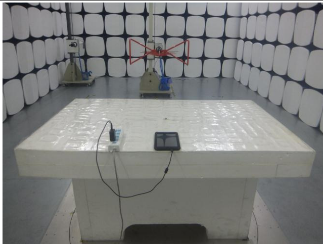
Conducted Emissions Test Setup Front View
