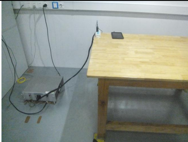
Conducted Emissions Test Setup Front View
