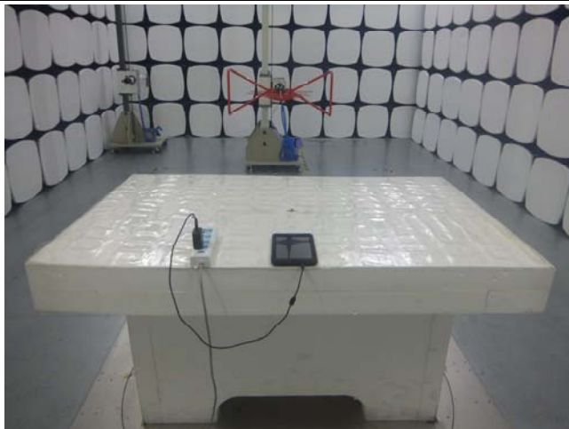
Radiated Spurious Emissions Test Setup Below 1GHz
