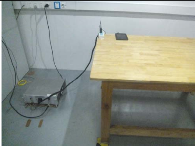
Conducted Emissions Test Setup Front View
