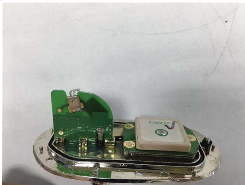
View of GSM/WCDMA Antenna
