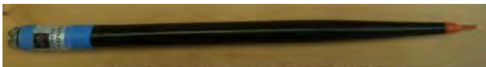
Figure 1 – MVG COMOSAR Dosimetric E field Dipole
