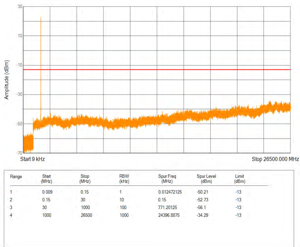
Band4 QPSK BW=5MHz Channel=19975 RB Size=25 Position=#0
