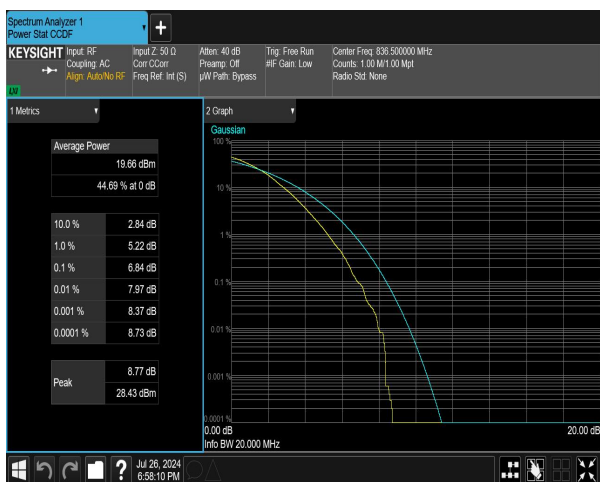
n5 SCS=15kHz DFT_256QAM BW=5MHz Channel=167300
