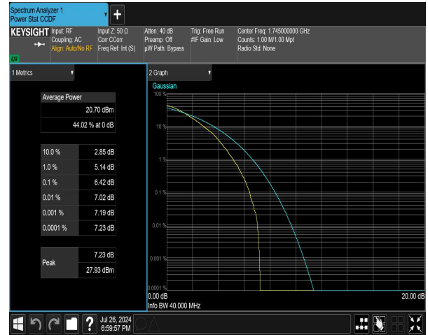
n66 SCS=15kHz DFT_64QAM BW=15MHz Channel=349000 RB=75@0 NVNT
