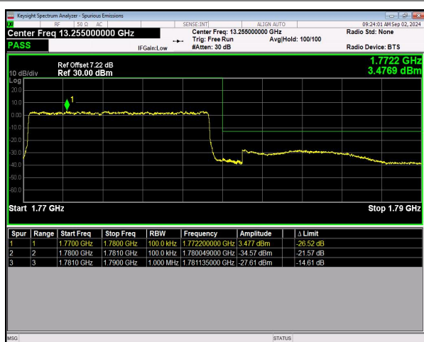
n66 SCS=15kHz DFT_BPSK BW=10MHz HighChannel=355000 RB=50@0 NVNT
