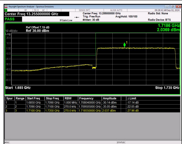
n66 SCS=15kHz DFT_64QAM BW=25MHz LowChannel=344500 RB=128@0 NVNT
