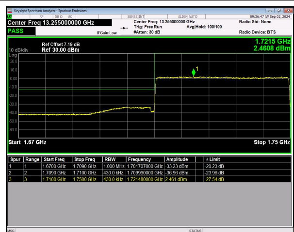
n66 SCS=15kHz DFT_16QAM BW=40MHz LowChannel=346000 RB=216@0 NVNT
