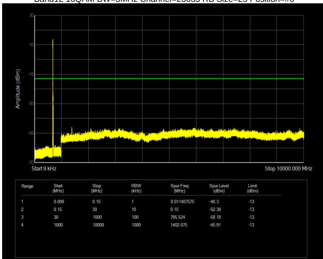
Band12 16QAM BW=5MHz Channel=23095 RB Size=25 Position=#0
