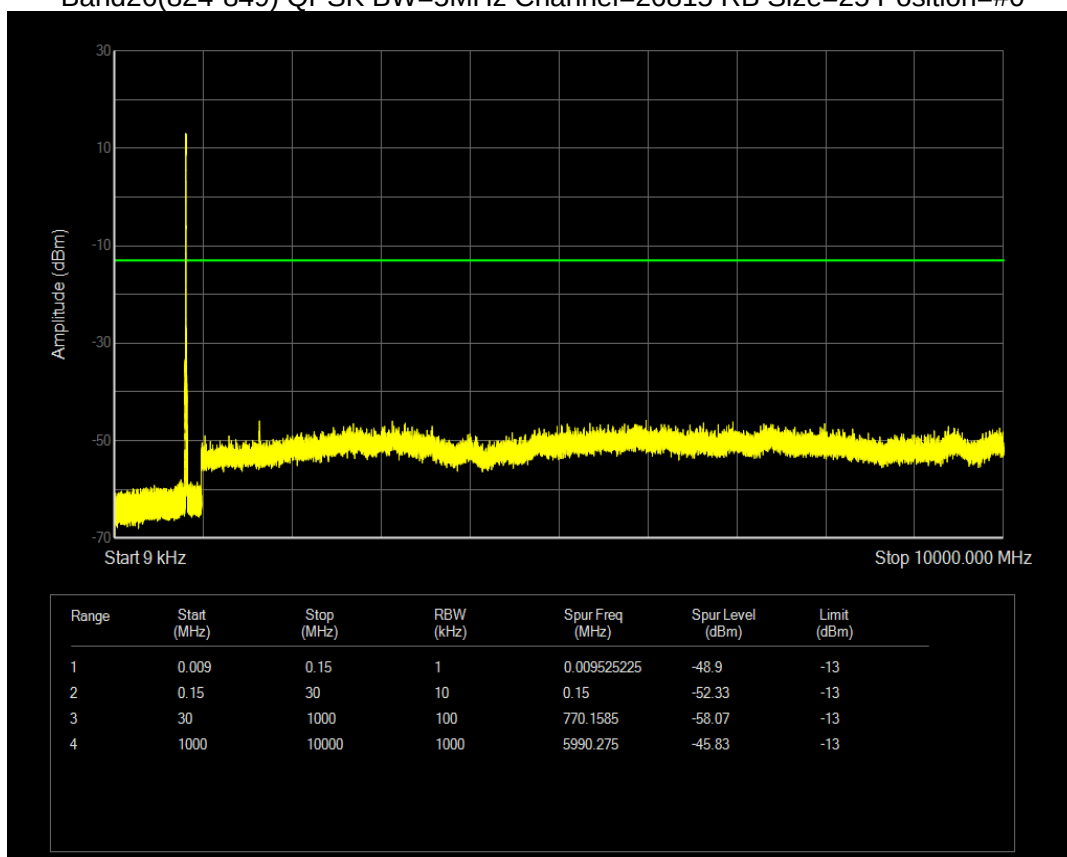
Band26(824-849) QPSK BW=5MHz Channel=26915 RB Size=25 Position=#0
