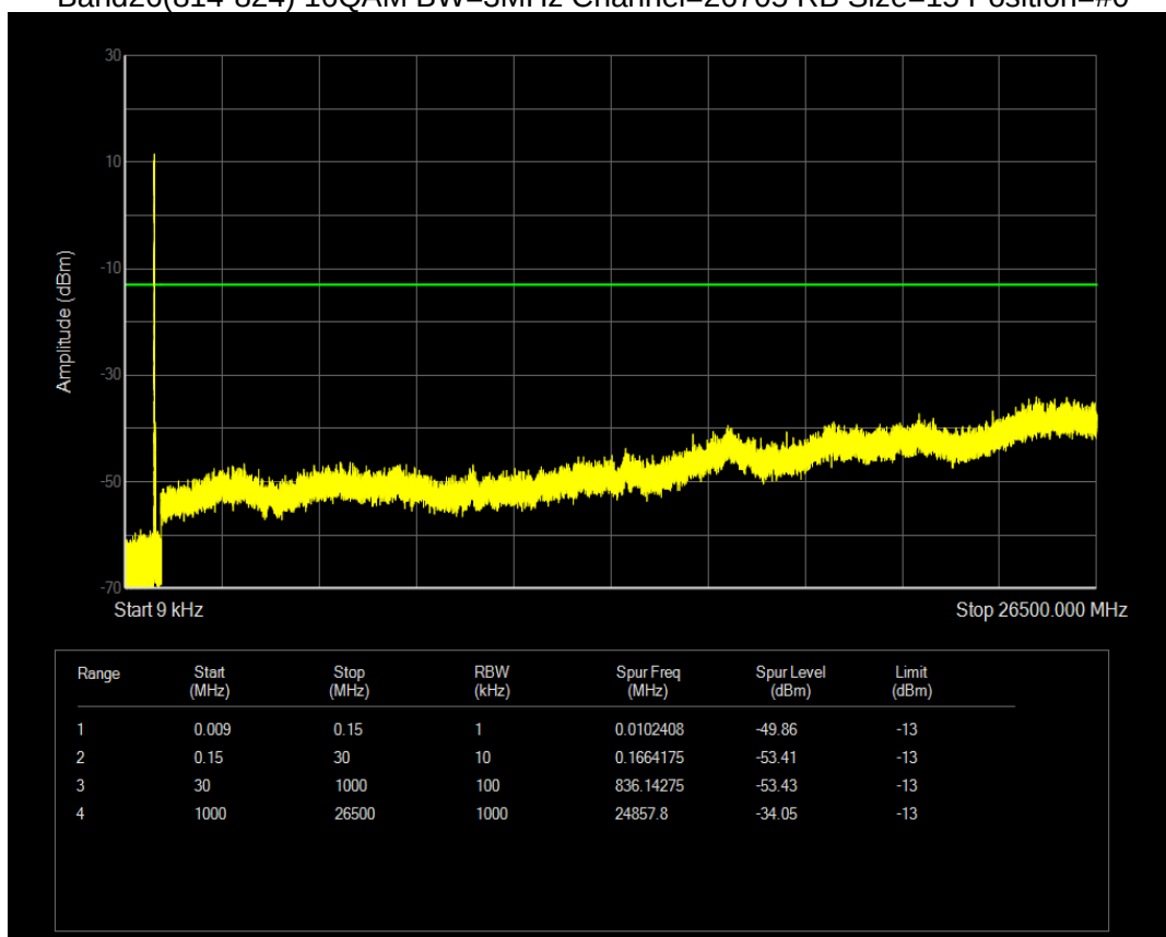
Band26(814-824) 16QAM BW=3MHz Channel=26740 RB Size=15 Position=#0
