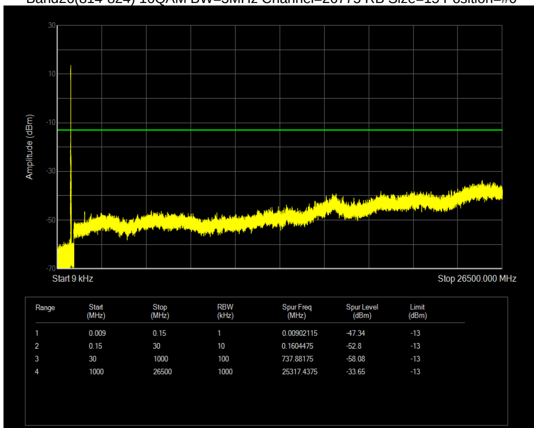
Band26(814-824) 16QAM BW=5MHz Channel=26715 RB Size=25 Position=#0
