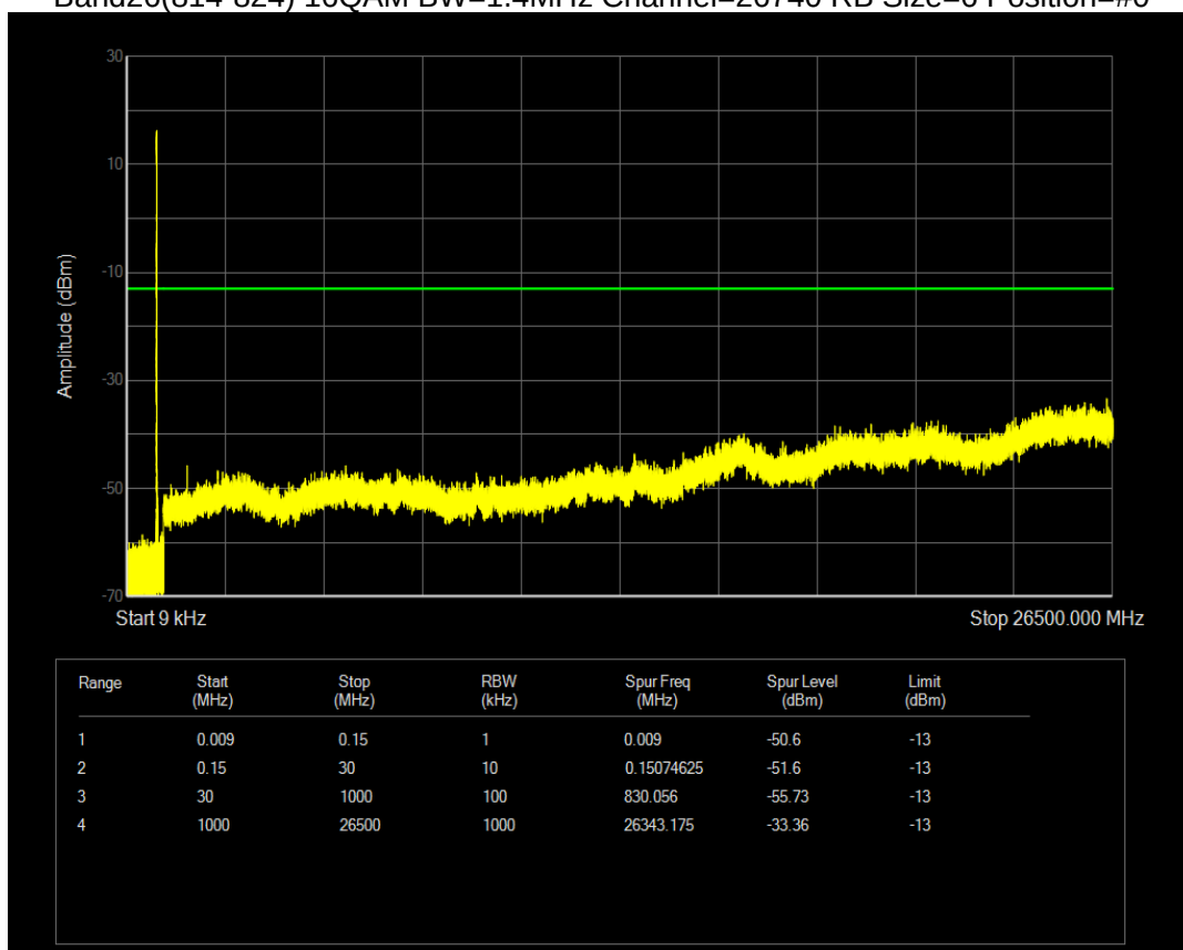
Band26(814-824) 16QAM BW=1.4MHz Channel=26783 RB Size=6 Position=#0
