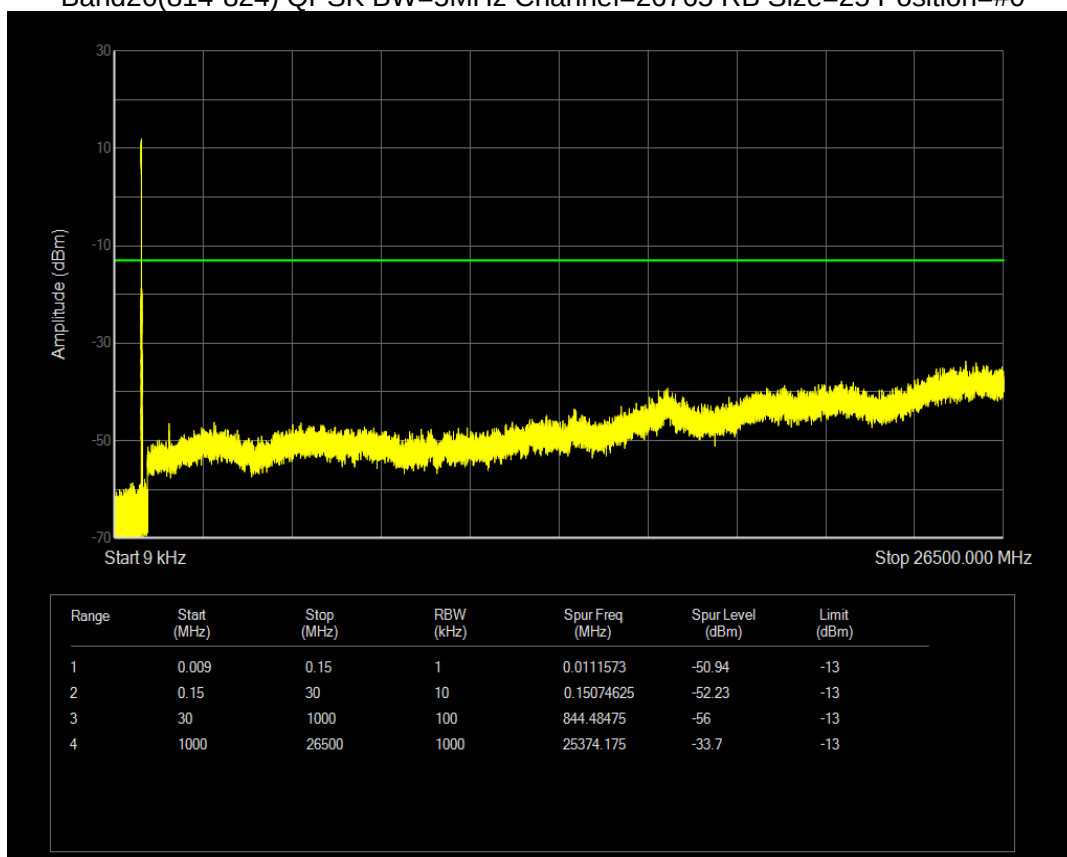
Band38 16QAM BW=10MHz Channel=37800 RB Size=50 Position=#0
