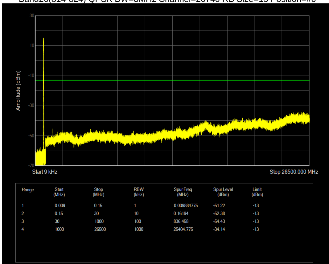
Band26(814-824) QPSK BW=3MHz Channel=26775 RB Size=15 Position=#0
