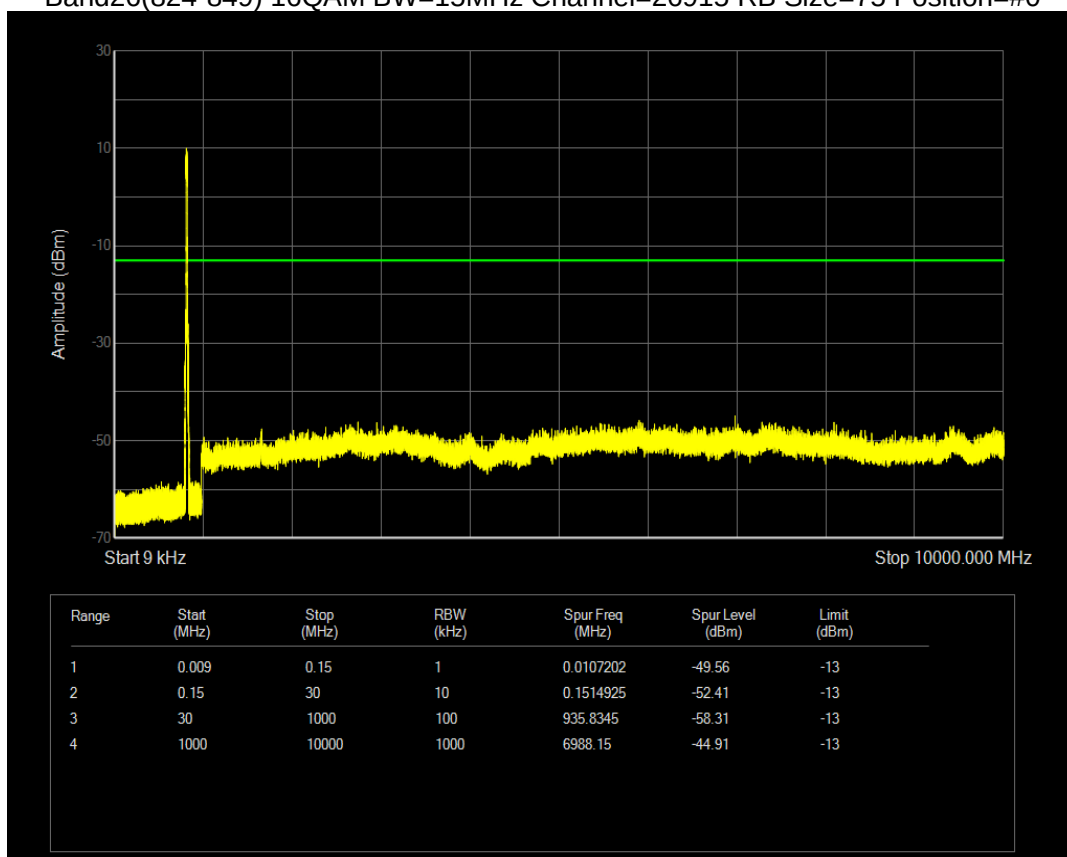
Band26(824-849) 16QAM BW=15MHz Channel=26965 RB Size=75 Position=#0
