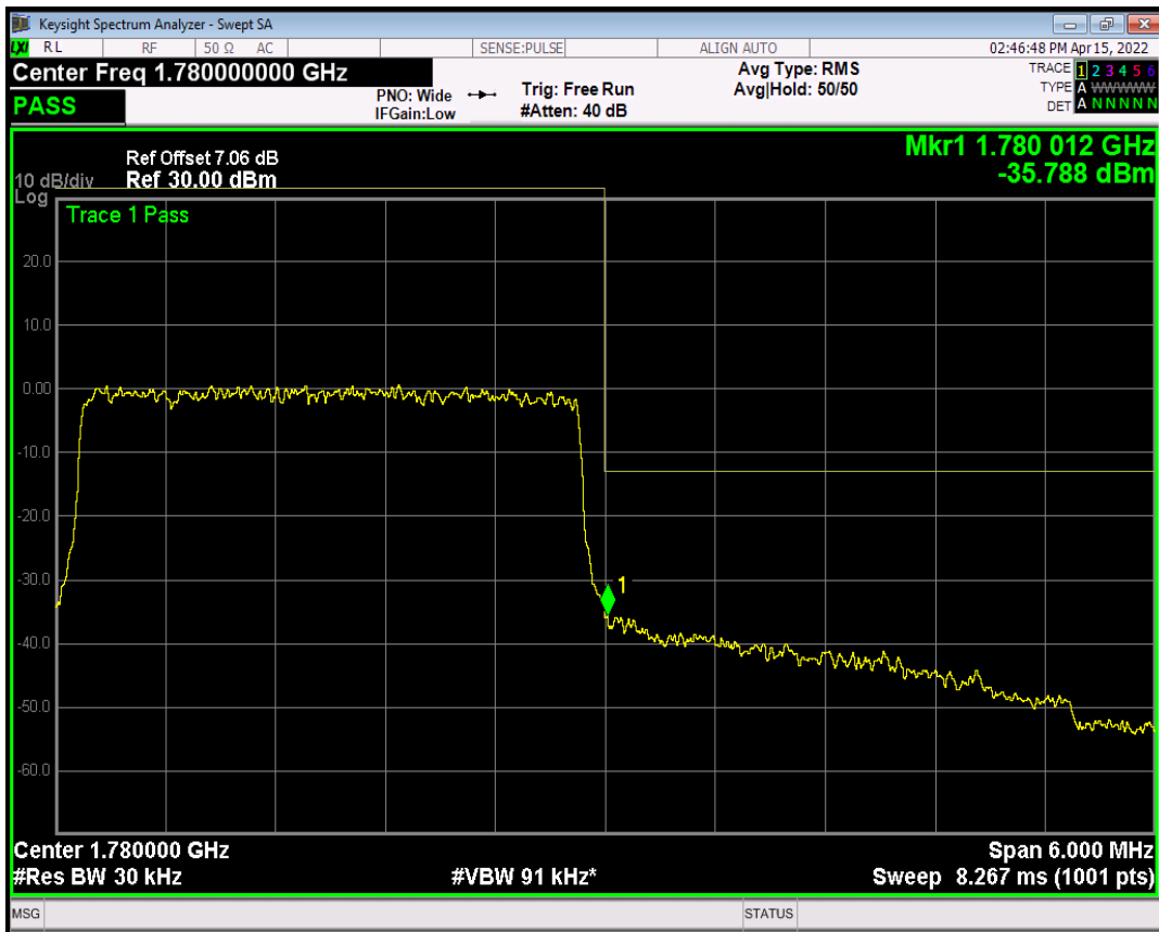
Band66 QPSK BW=5MHz Channel=131997 RB Size=25 Position=#0
