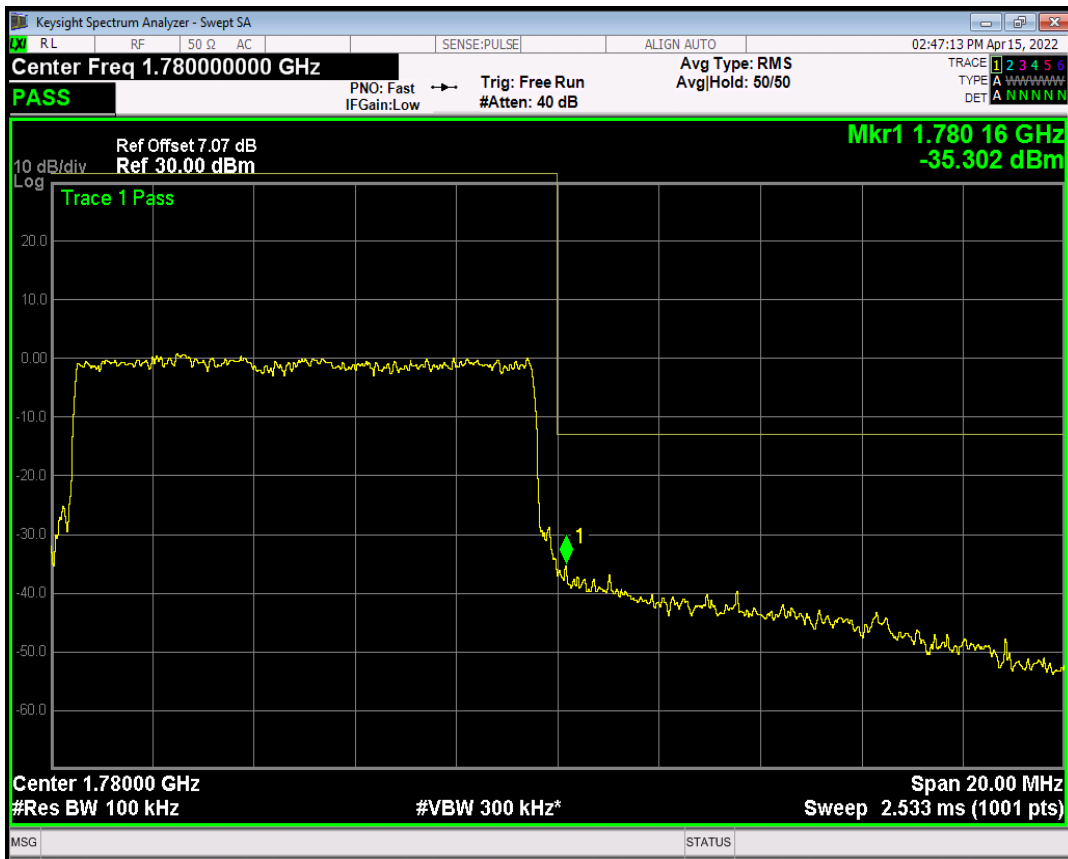
Band66 QPSK BW=15MHz Channel=132047 RB Size=75 Position=#0
