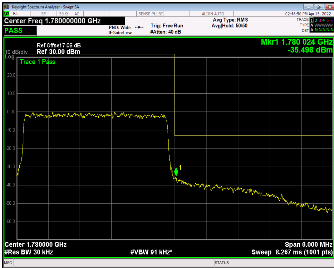
Band66 QAM16 BW=5MHz Channel=131997 RB Size=25 Position=#0
