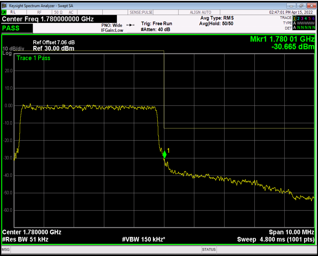
Band7 QAM16 BW=10MHz Channel=20800 RB Size=50 Position=#0
