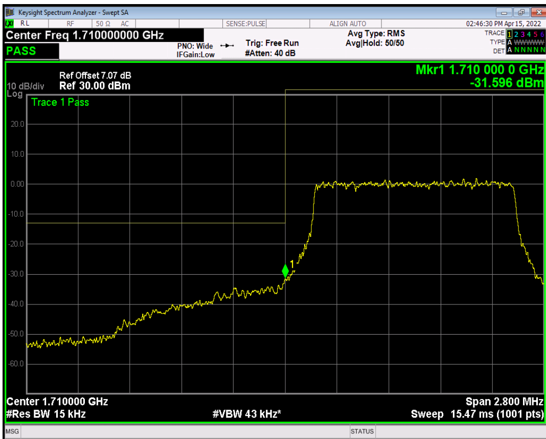
Band66 QPSK BW=1.4MHz Channel=132665 RB Size=6 Position=#0
