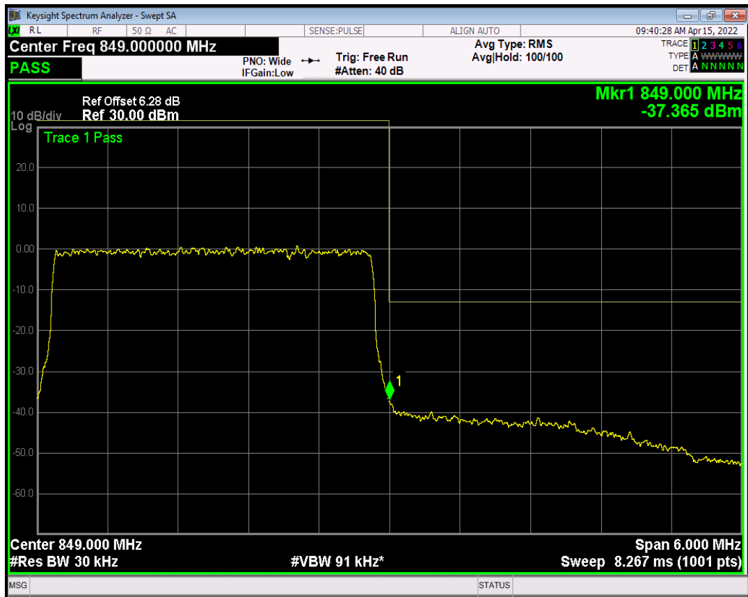
Band5 QAM16 BW=5MHz Channel=20425 RB Size=25 Position=#0
