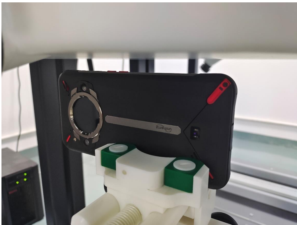
Body Left side (separation distance is 10mm)
