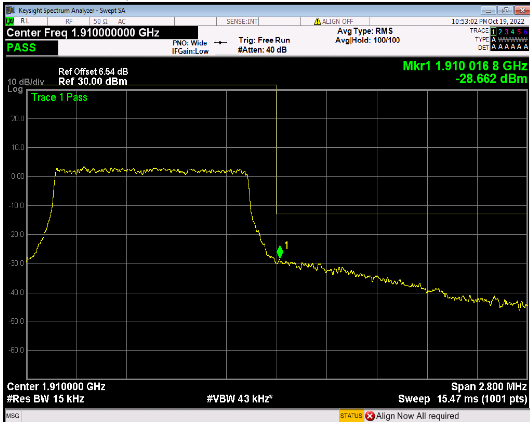
Band2 16QAM BW=10MHz Channel=18650 RB Size=50 Position=#0
