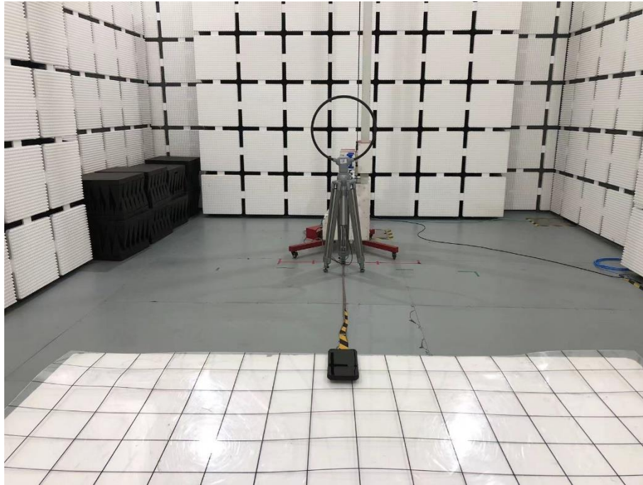
Radiated Spurious Emission Test Setup Photo - Below 1GHz
